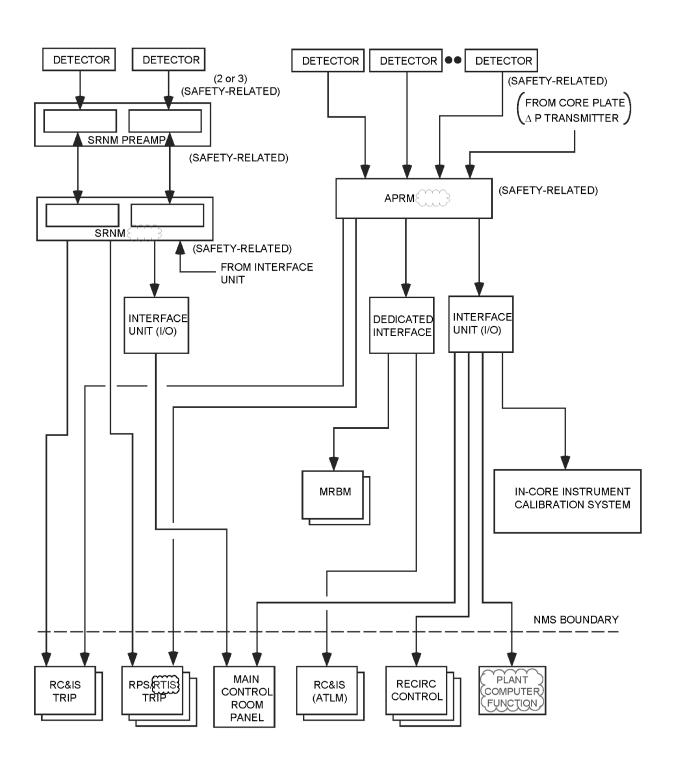
Figure 7.6-4a Basic Configuration of a Typical Neutron Monitoring System Division
