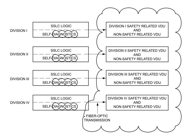
Figure 7.1-1 SSLC Self-Test System Diagnosis
