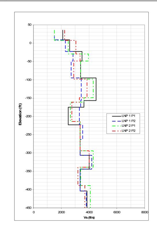
Note: Profiles LNP 1 P1 and LNP 2 P1 are based on suspension logging data Profiles LNP 1 P2 and LNP 2 P2 are based on downhole data
