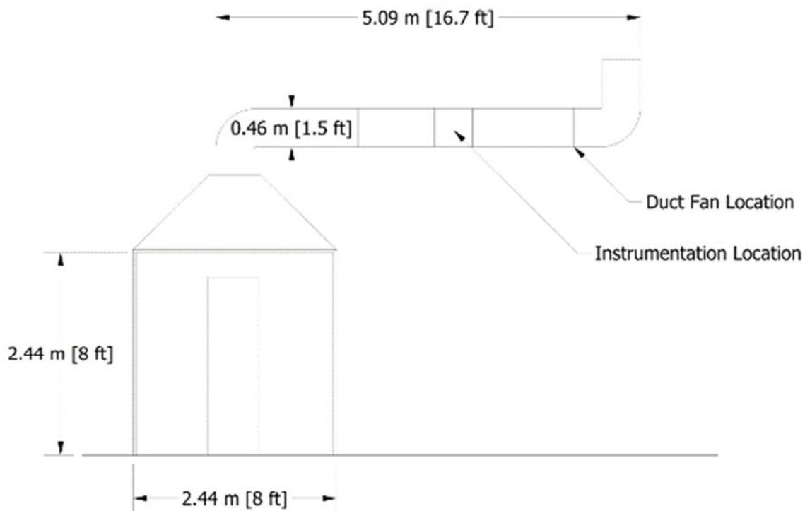
Figure 4-1. Schematic diagram of the small calorimeter.
