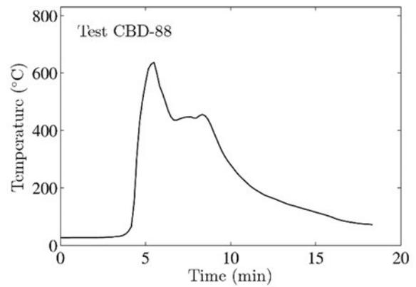
Figure A-15. Enclosure temperatures, Tests 83-88.
