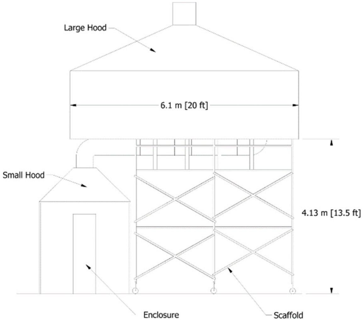
**Figure 4-2. Schematic diagram of the small calorimeter underneath the large hood at the CBD test facility.**
