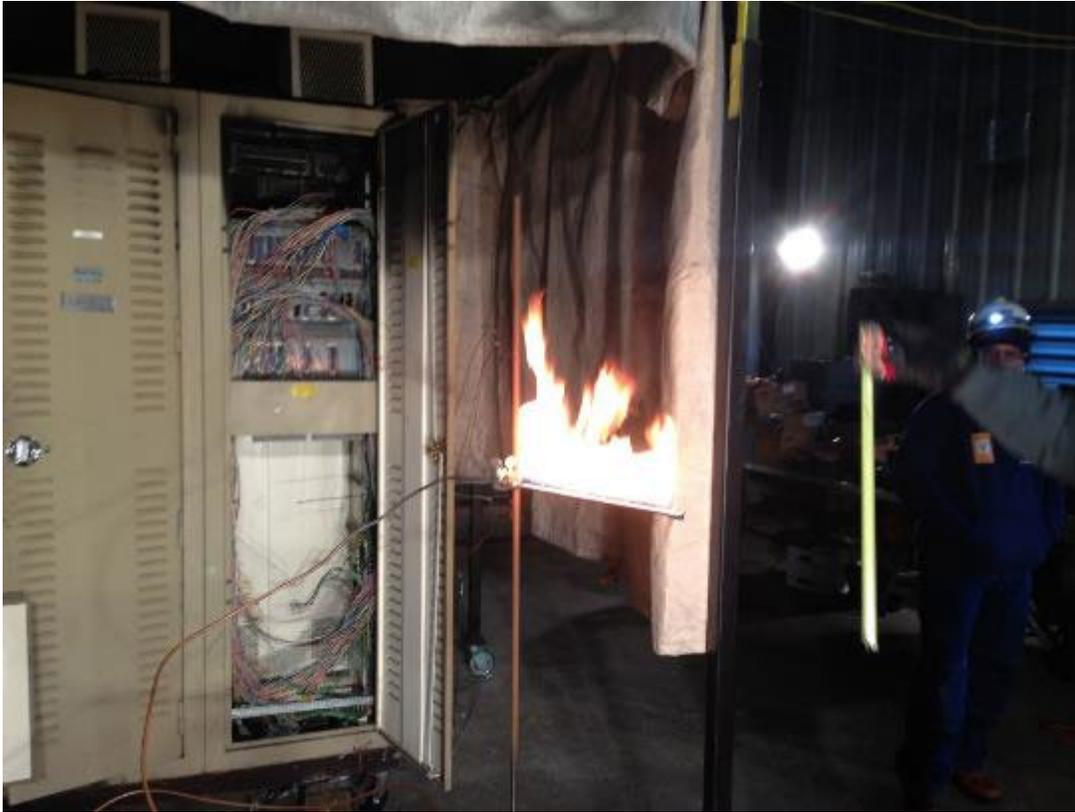
**Figure 4-4. Photograph of 30 cm (12 in) propane line burner.**
