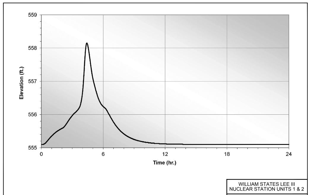
Flood Elevation Hydrograph Make-Up Pond A 6-Hour Local Intense Precipitation
