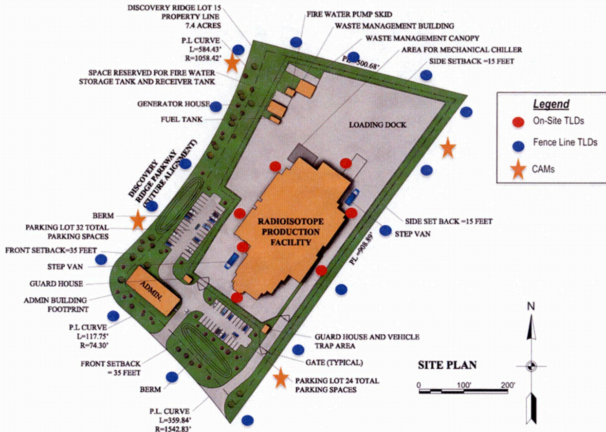
Figure 11-6. Location of On-Site Environmental Thermoluminescent Dosimeters and Continuous Air Monitors
