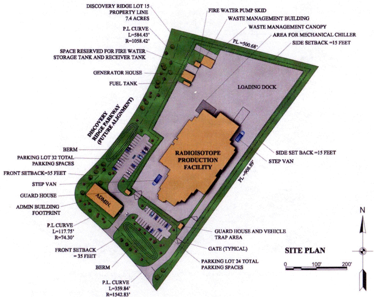
Figure 1-4. Radioisotope Production Facility Site Layout
