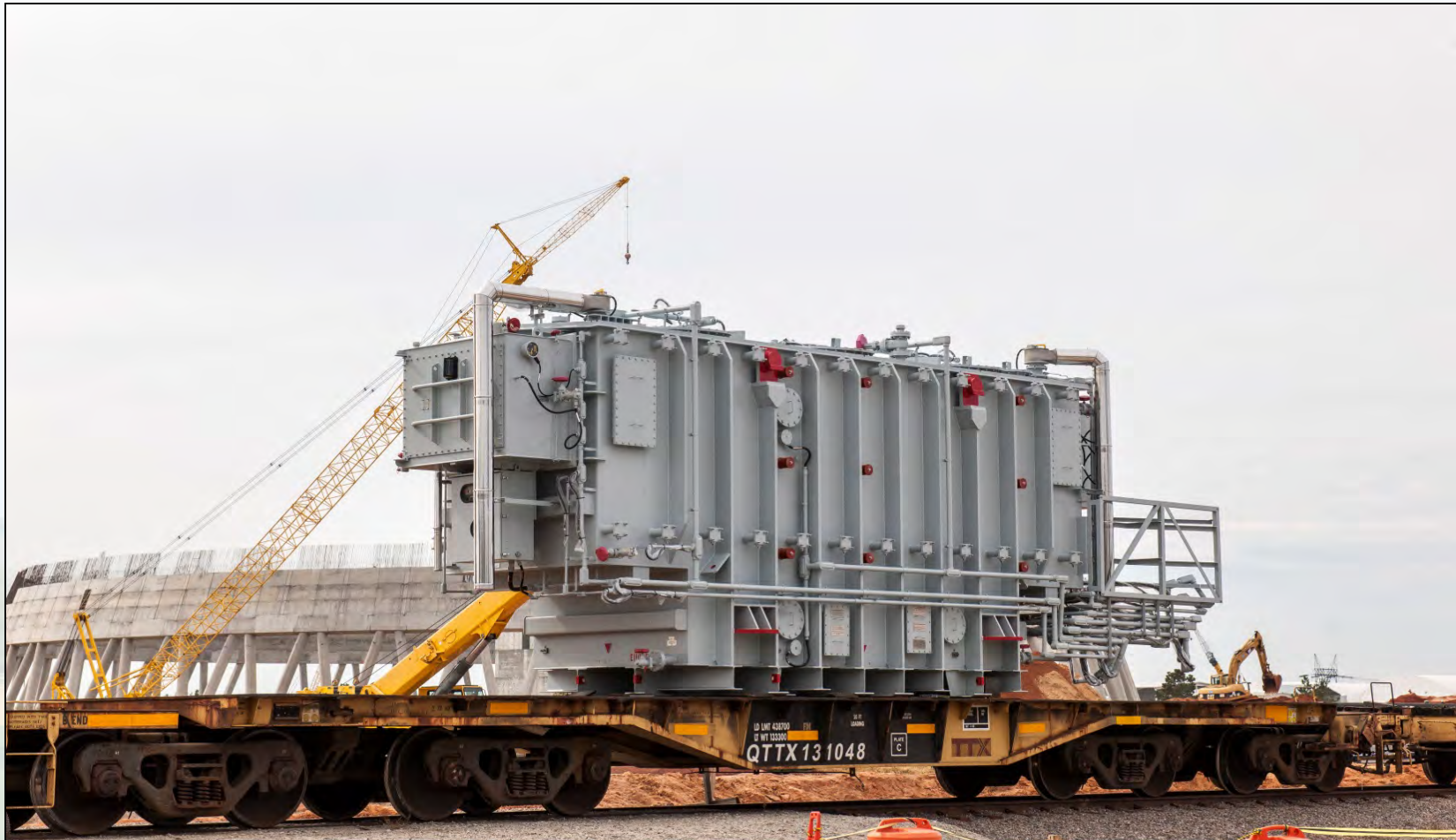
Vogtle Unit 4 reserve auxiliary transformer.
