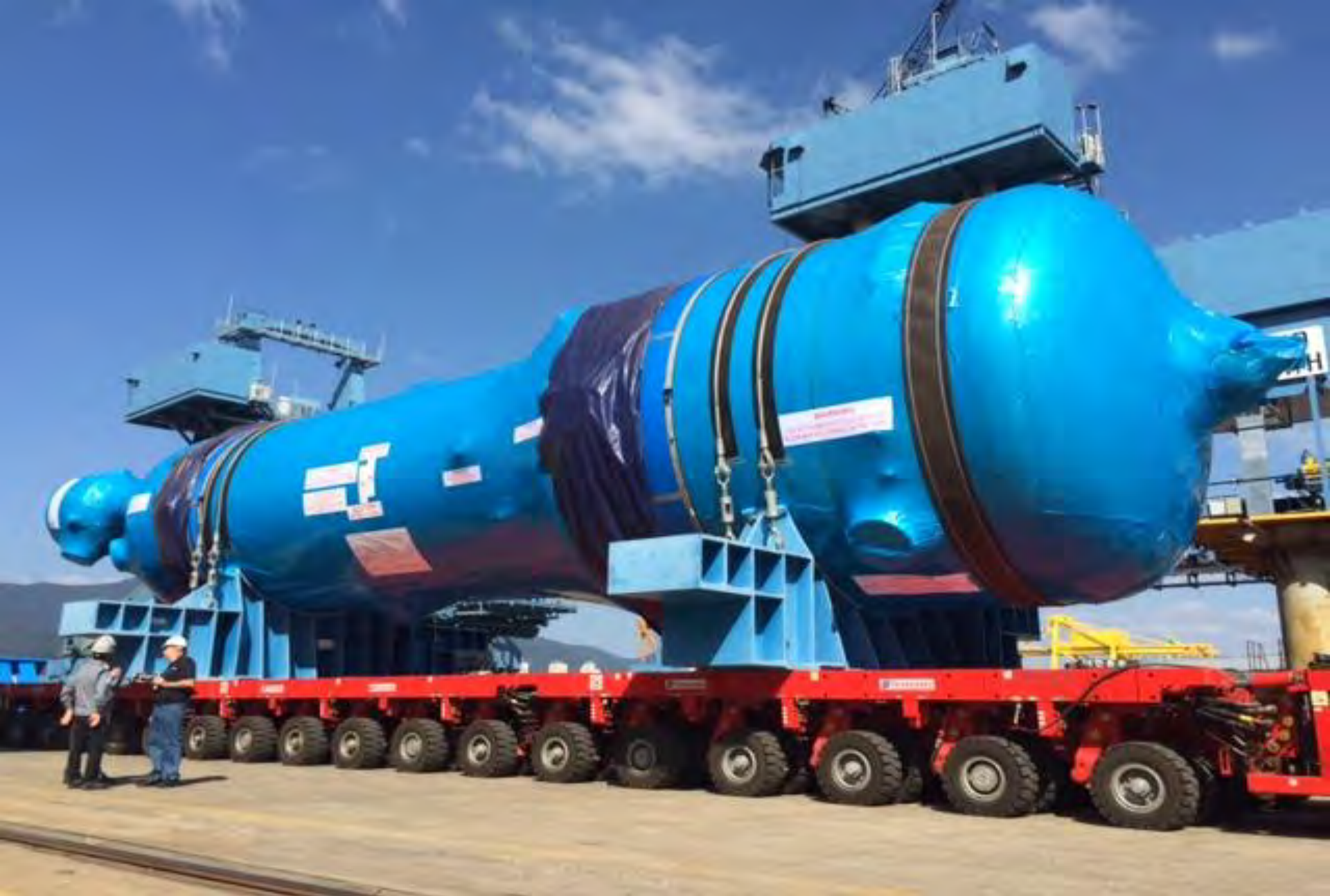
Steam Generator Load Out
