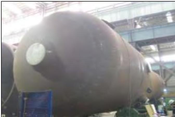
Hydro test Complete for Unit 2A SG
