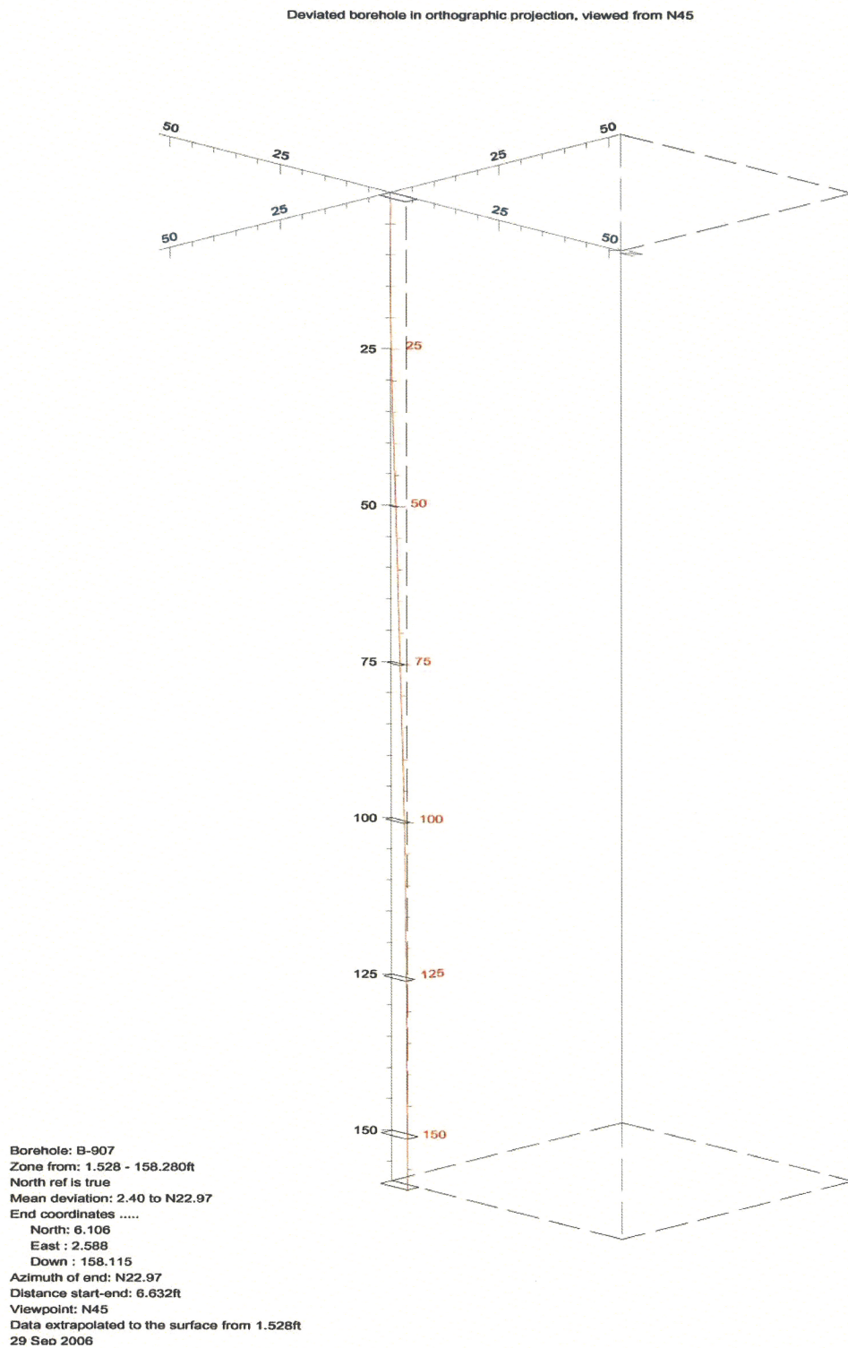
Figure 14. Boring B-907, Deviation Projection (dimensions in feet)
