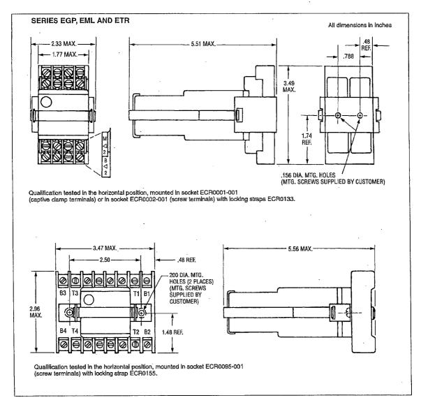
Series EGP, EML and ETR AGASTAT® control relays must be mounted in the horizontal position; performance specifications of these units are valid only when they are mounted as indicated in either of the above drawings.
