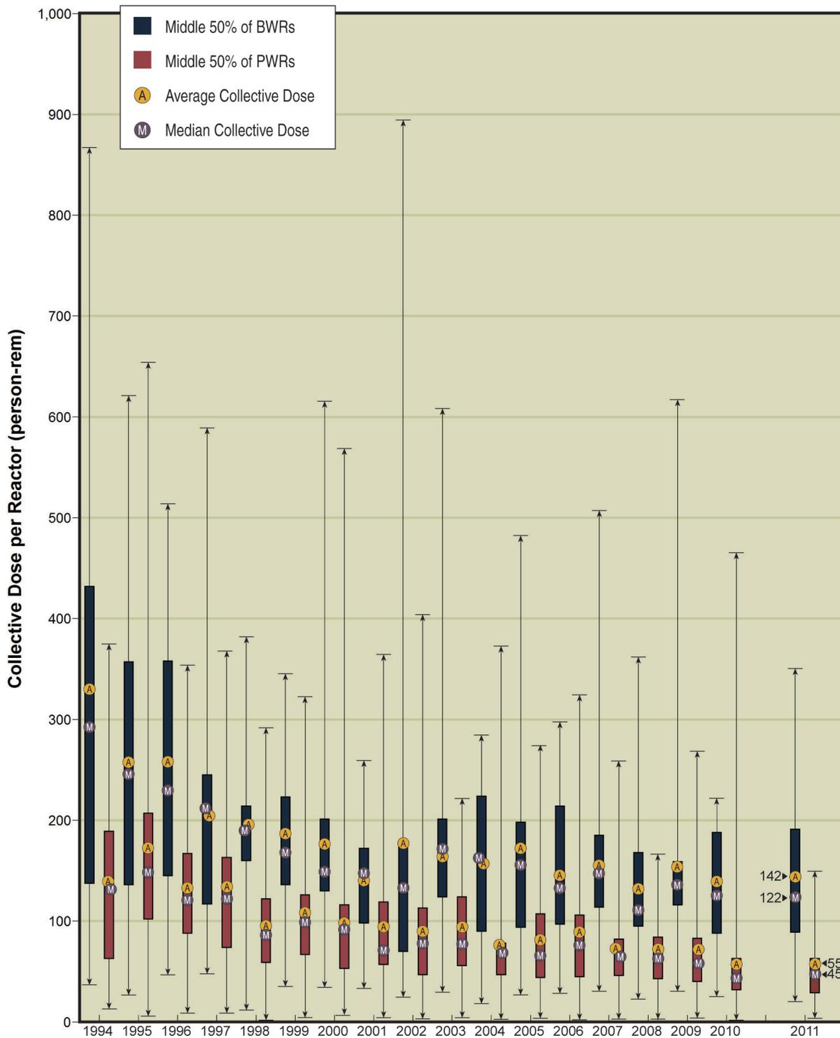
Figure 4.4. Average, Median, and Extreme Values of the Collective Dose per Reactor 1994–2011
