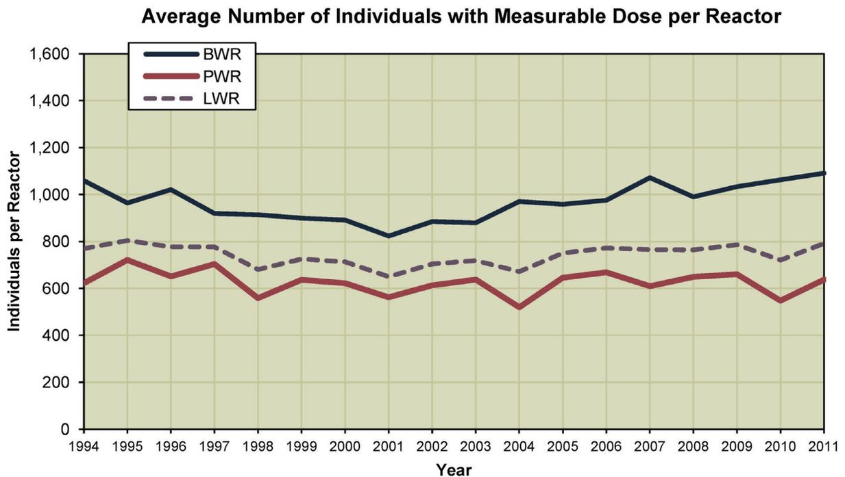
**Figure 4.1.** Average Collective Dose per Reactor and Average Number of Individuals with Measurable Dose per Reactor 1994–2011
