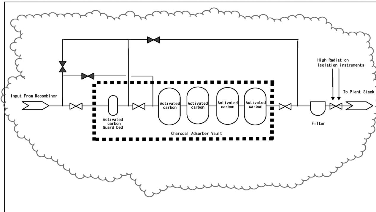
Figure 15.7-2 Offgas System (See Subsection 11.3)
