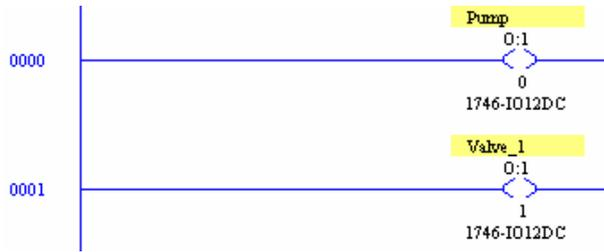
When does the pump come on? - When the START\_PB is pressed. When does Valve 1 open? - Only while the pump is running and then only when the LOW level is reached:
