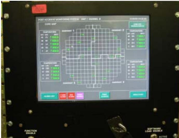
**Figure 2-55 Westinghouse Common Q Qualified Flat Panel Display**
