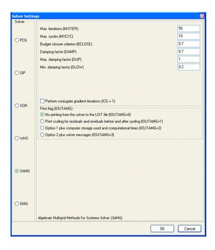
The SAMG solver has advantages over other solvers included with Visual MODFLOW for problems with large grids or a highly variable hydraulic conductivity field. The solver is also less sensitive to the initial head distribution (Reference 2.4.12-C-1).
