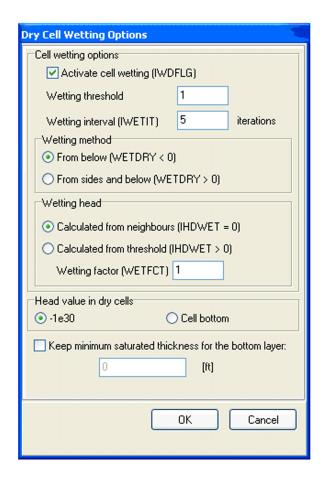
The discontinuity of the strata in the top four layers of model produces cyclic wetting and drying of cells in the areas where steep changes in layer elevations and stratigraphic layer pinch outs occur. This cyclic wetting and drying interferes with numerical convergence by the solver. By increasing the wetting interval, the solver can converge on a solution. A recommended range for the wetting interval is between three and five iterations (Reference 2.4.12-C-13)
