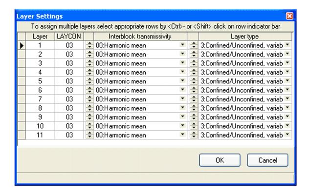
The MODFLOW default method for assigning inter-block transmissivity using the harmonic mean is used for all layers.
