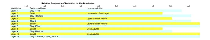
The relative frequencies of detection of the units indicate continuity or lack thereof for each geotechnical layer.
