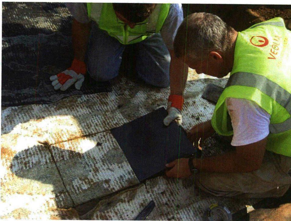
Fig. M. 17. GCL sample with cut perimeter prior to sliding of sampling plate and removal.
