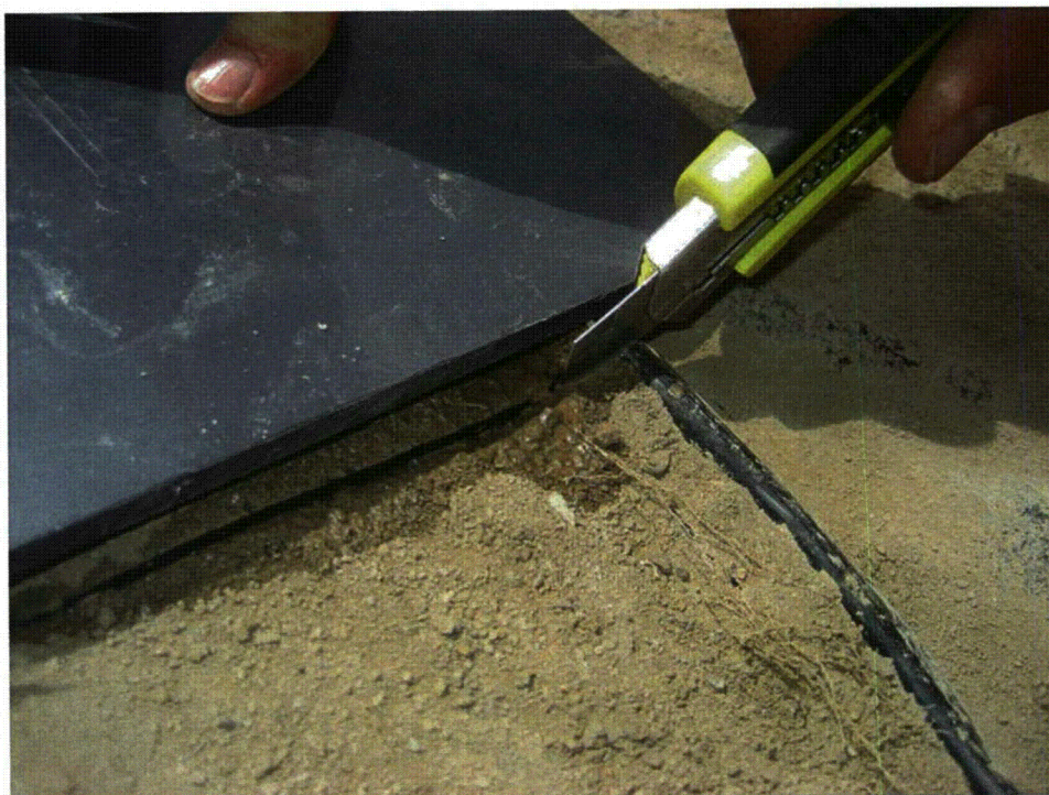
Fig. M. 22. Moisture seeping from GM while cutting through GM patch in Test Pit 1.
