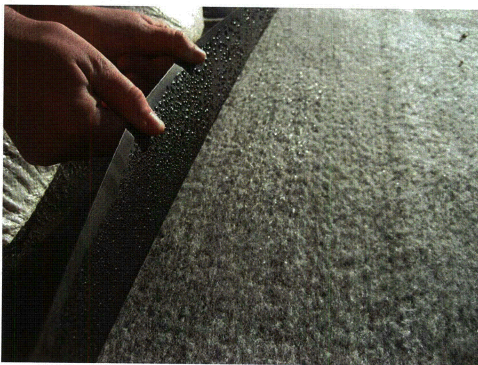
Fig. M. 26. Condensation on GM overlying GCL underside from solar heating.
