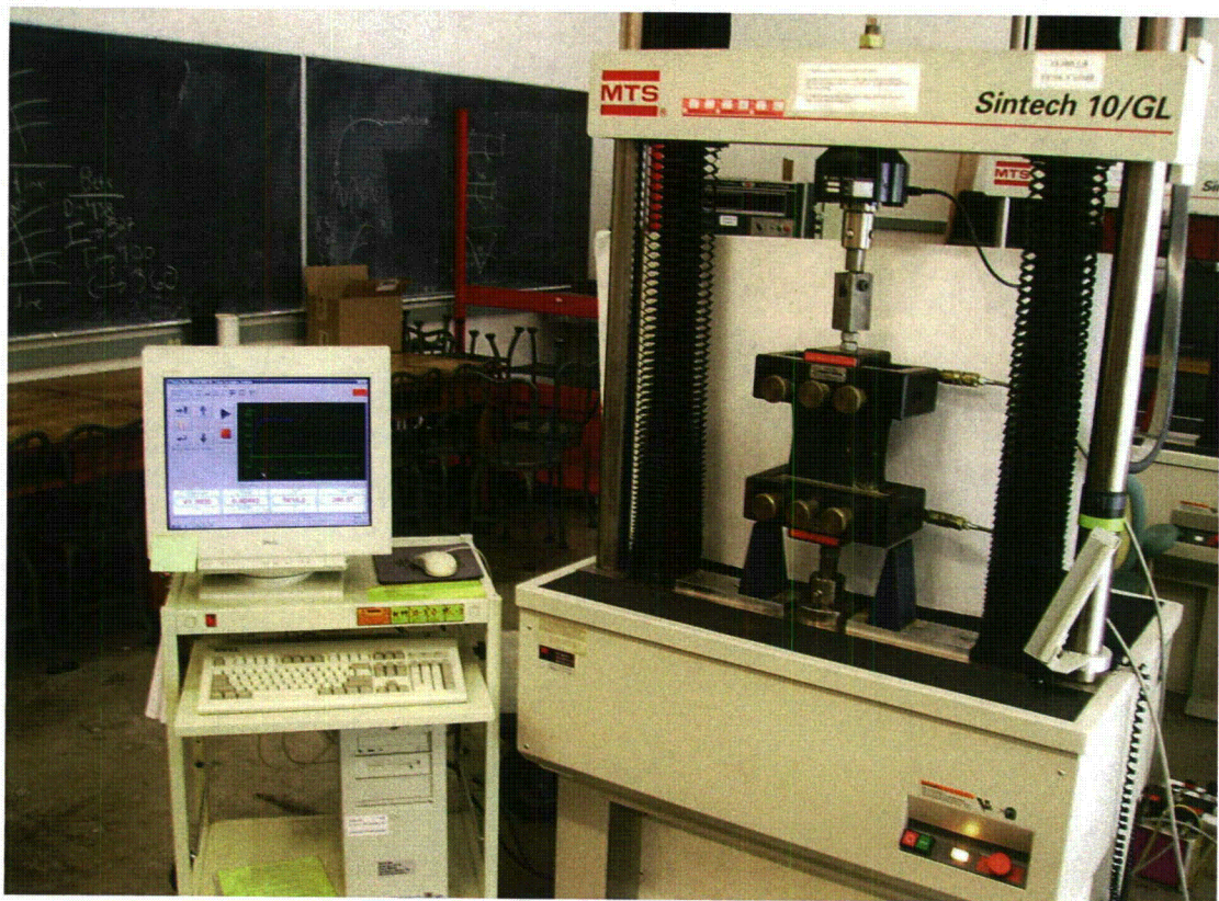
Fig. Q1.MTS Sintech 10/GL load frame equipped with Curtis Geo-Grips used for tensile testing.
