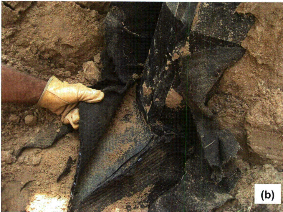
Fig. M. 14. Examples of seams observed during exhumation: (a) dual-track wedge weld and (b) extrusion well to boot for gas well near Test Pit 4.
