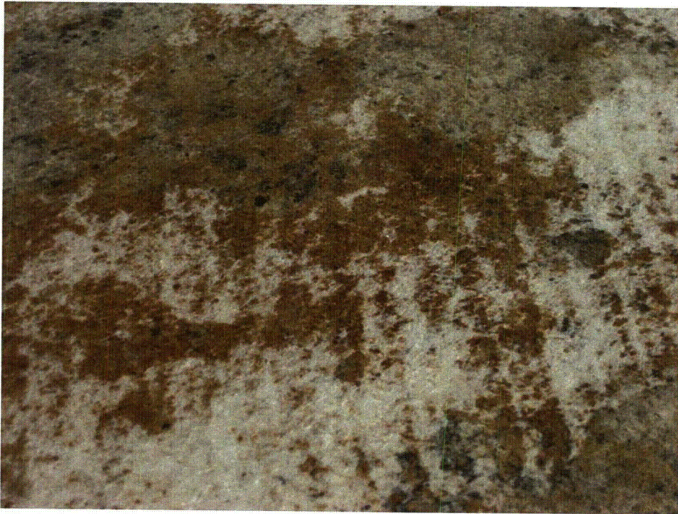
Fig. M. 16. Staining on GCL carrier nonwoven geotextiles.
