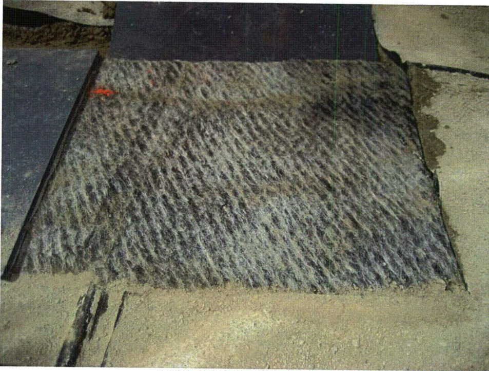
Fig. M. 23. Moisture visible on GCL after rupturing GM patch in Test Pit 1.
