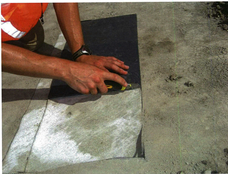
Fig. M. 21. Cutting of GCL sample perimeters in Test Pit 2. Staining visible on GCL carrier geotextiles.
