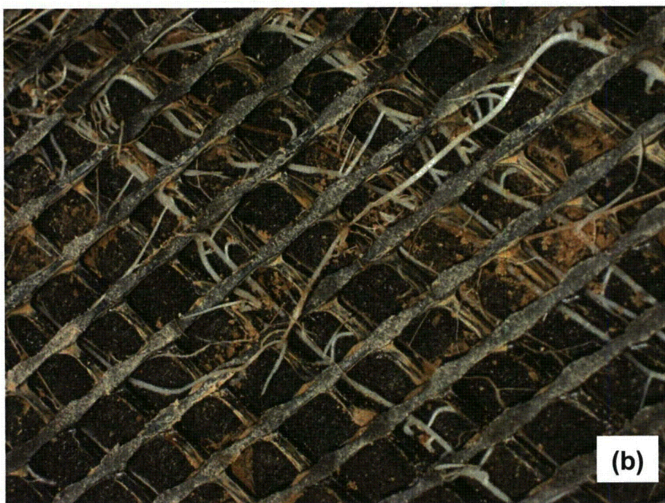
Fig. M. 13. Roots in the GDL and fines coating the ribs of the geonet in Test Pit 1: (a) overview and (b) close up.
