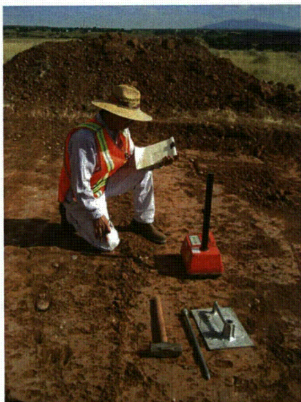
Fig. A.80. Measuring in-situ density prior to sampling.
