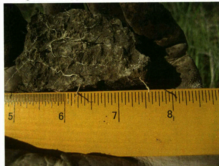
Fig. A.73. Root planes visible on ped removed from bottom of desiccated CCL.
