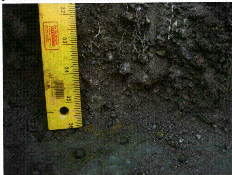
Fig. A.72. Roots visible down to veg. barrier in all profiles.
