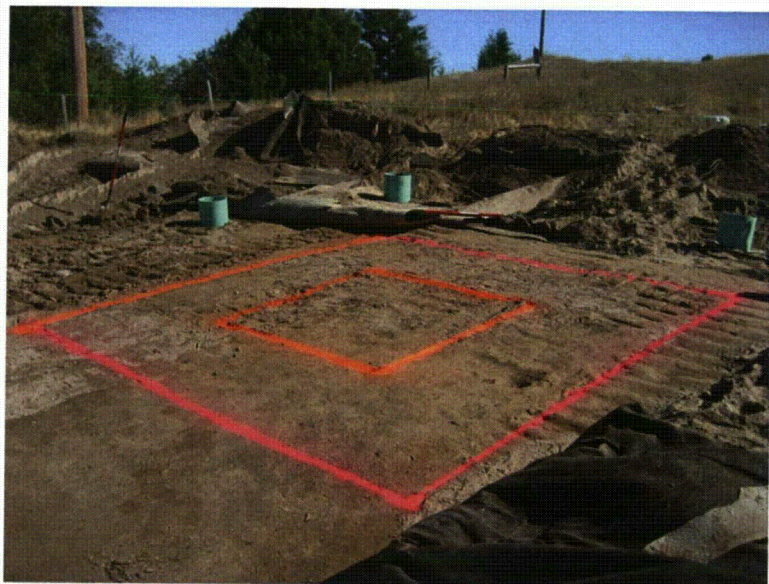
Fig. A.28. Installing SDRI under GM into CCL.
