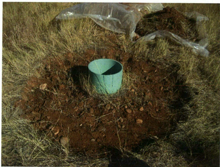
Fig. A.92. Excavating additional soil during sampling.
