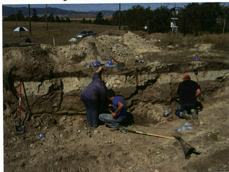
Fig. A.34. Sampling ET cover for water content profile.
