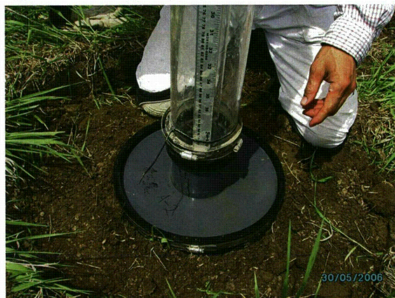
Fig. A.45. Installing Mariette bottle for constant head testing.
