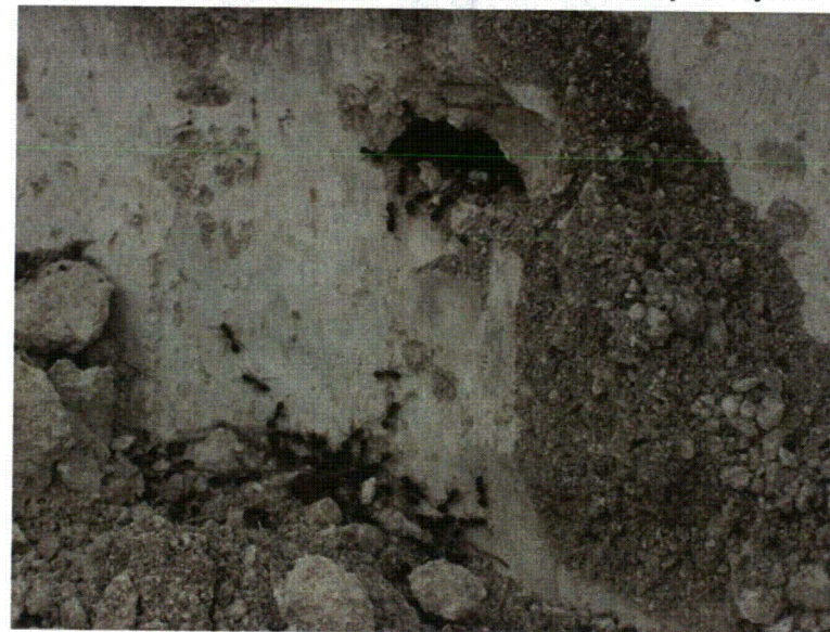
Fig. A.23. Close-up of macroscopic in-situ flow path.
