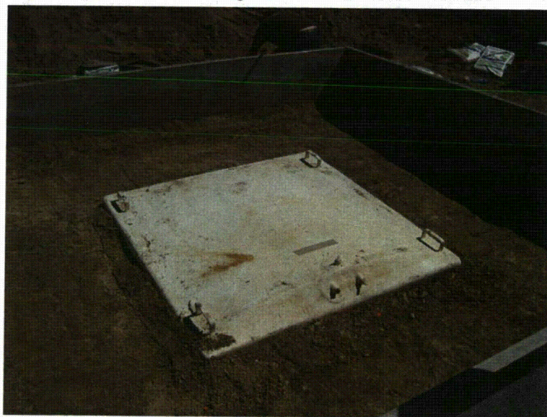
Fig. A.30. SDRI inner ring after assembly but prior to filling.
