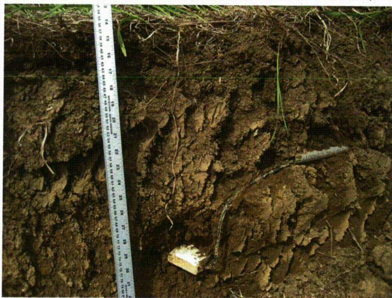
Fig. A.49. In-situ water content reflectometer.
