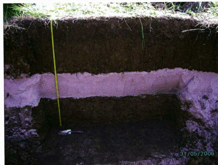
Fig. A.54. AO1 (Capillary barrier) cover profile.
