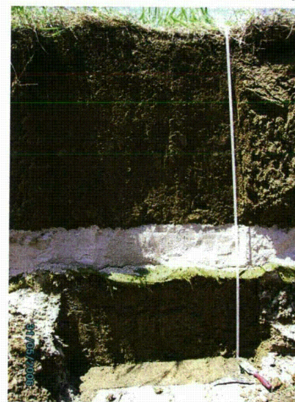
Fig. A.58. AO2 (Capillary barrier) cover profile.
