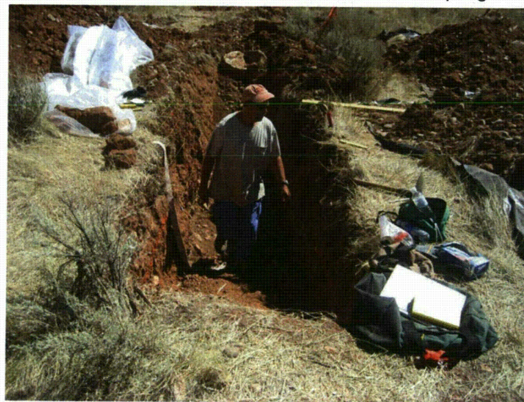
Fig. A.95. Trench for examination of soil structure.
