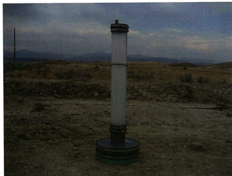
Fig. A.15. Constant head TSB in operation.
