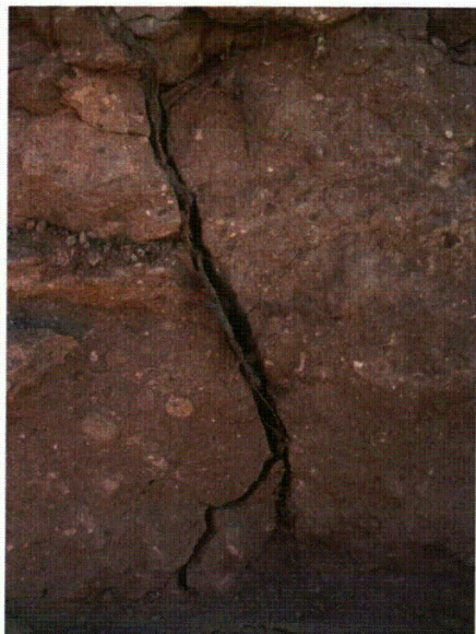
Fig. A.36. Failure along vertical root planes during trenching.
