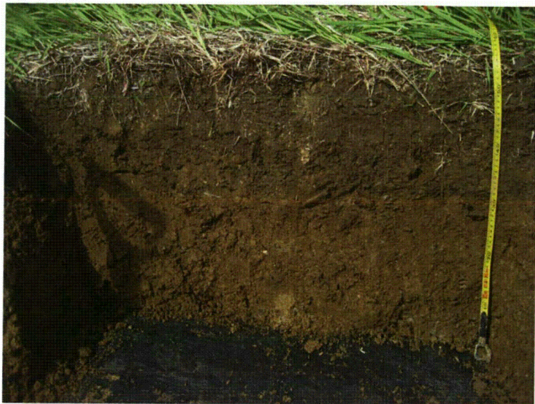
Fig. A.47. Conventional cover profile (soil above GM).
