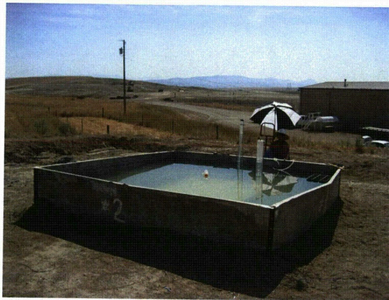
Fig. A.19. Operating SDRI with constant head inner ring.
