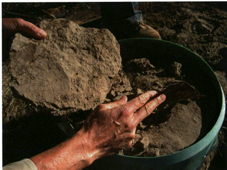
Fig. A.26. Horizontal plane of roots found during block sampling.
