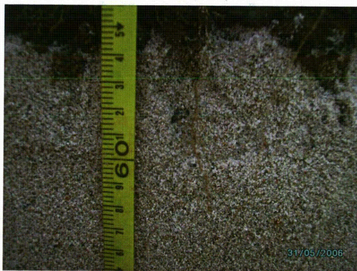
Fig. A.57. Close-up of undisturbed roots extending across capillary barrier and into course layer in AO1.
