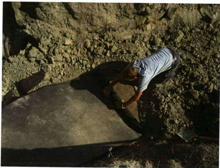
Fig. A.18. Removing lysimeter GDL for laboratory analysis.
