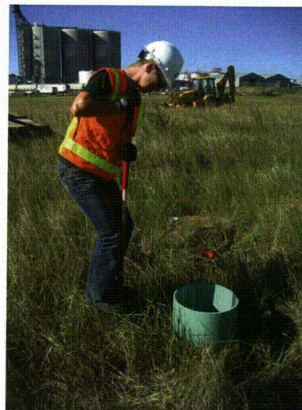
Fig. A.67. Digging block sample for laboratory analysis.
