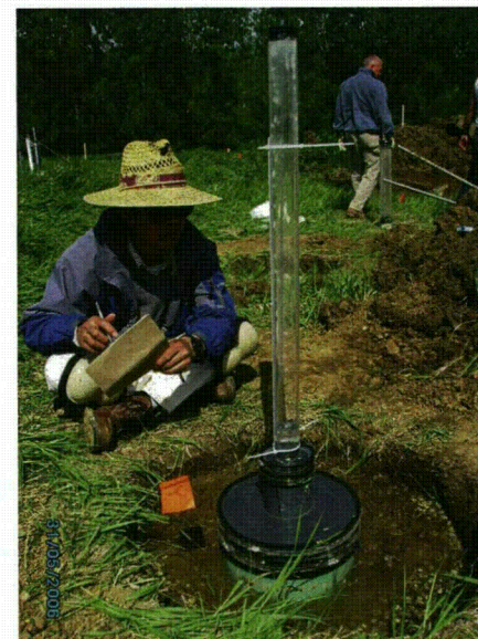
Fig. A.46. TSB data collection with narrow Mariette bottle.
