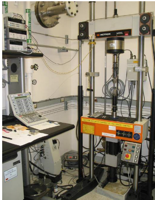
Figure 3-1 Test Sample Pre-Cracking Station. This Instron load frame can be used to pre-crack a specimen prior to inserting the specimen into a CGR test system. Leads for dcpc attach to a sample and to the electronics in the upper-left corner of the picture.
