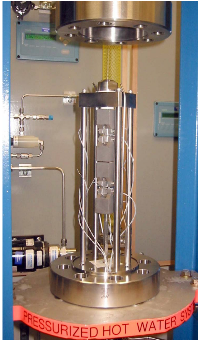
Figure 3-8 Two CT Samples Mounted in Series Prior to SCC Crack-Growth Testing. The bright, non-oxidized autoclave load train indicates first usage of this test system.
