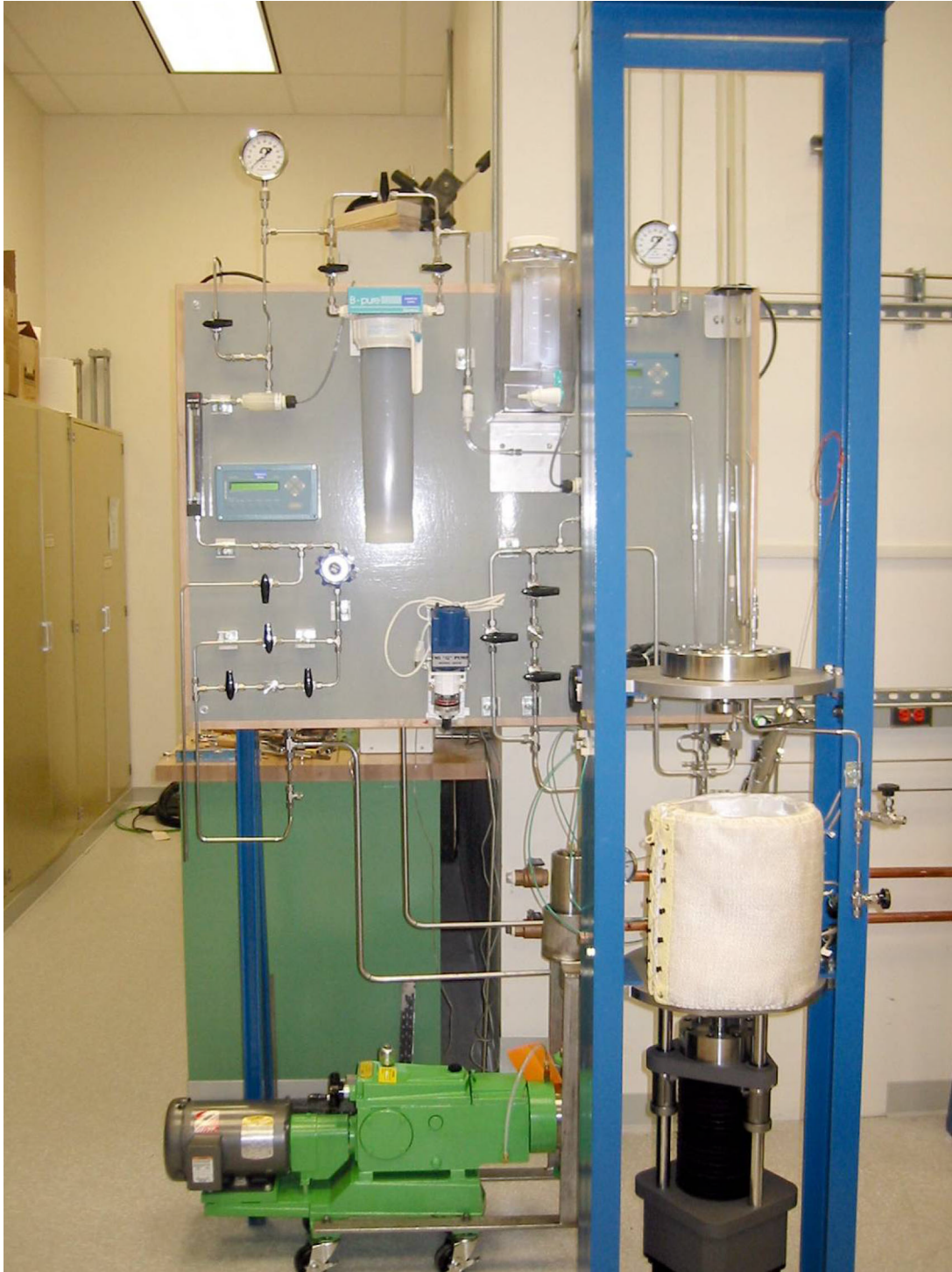
Figure 3-4 Crack-Growth Test System #1 when it was Near Completion and Before the Initial Shakedown Test. Green item on floor is the high-pressure (3000 psi) pump. Off-white jacket is the heating blanket that surrounds the autoclave lid (not shown). Blue frame is the load frame.
