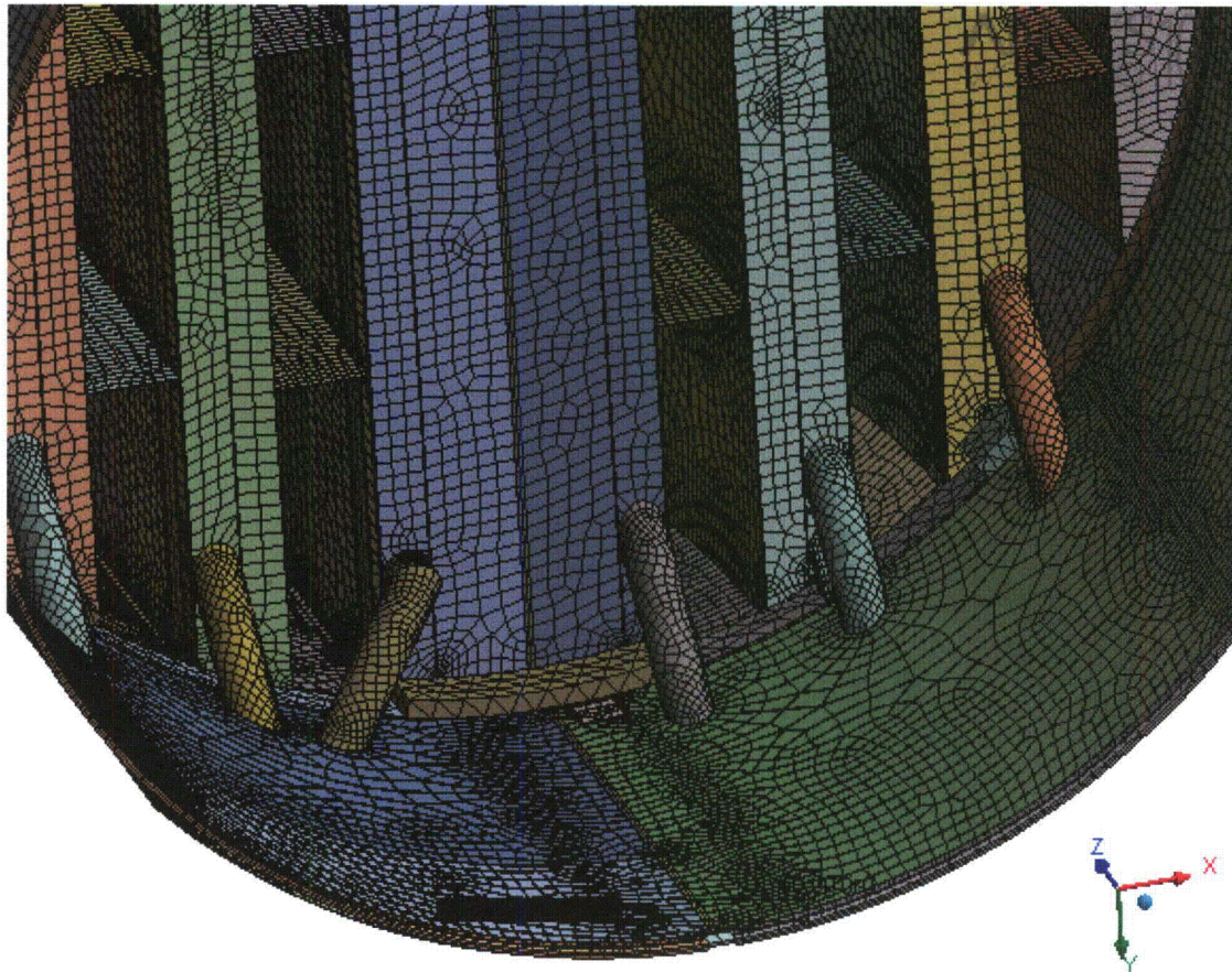
Figure 9c. Close up of mesh showing drain pipes and hood supports.
