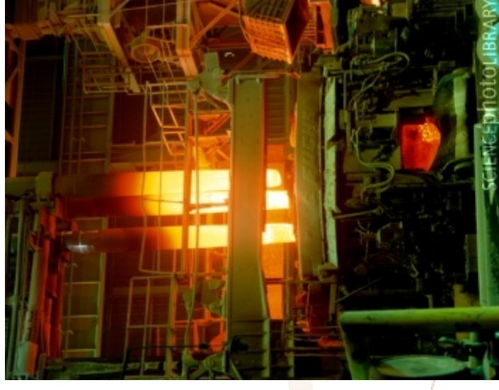
Figure 3. Three graphite electrodes glow red hot after their removal from an electric arc furnace used to produce steel.
