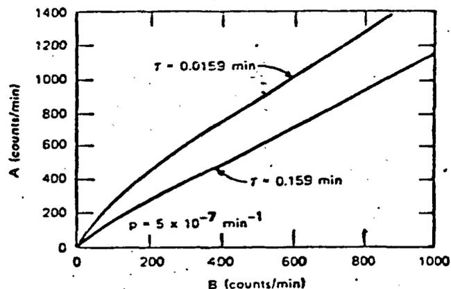
Fig. 1 Effect of background on the optimum alarm set point.
