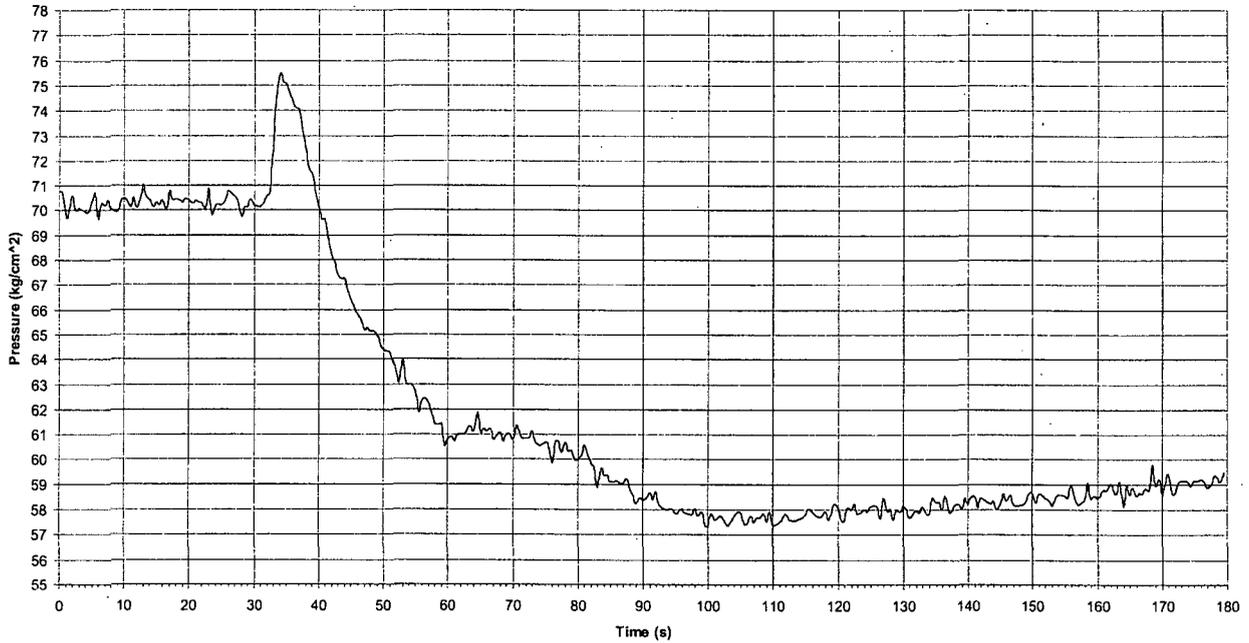
**Figure 3 Steam dome pressure (plant data)**
