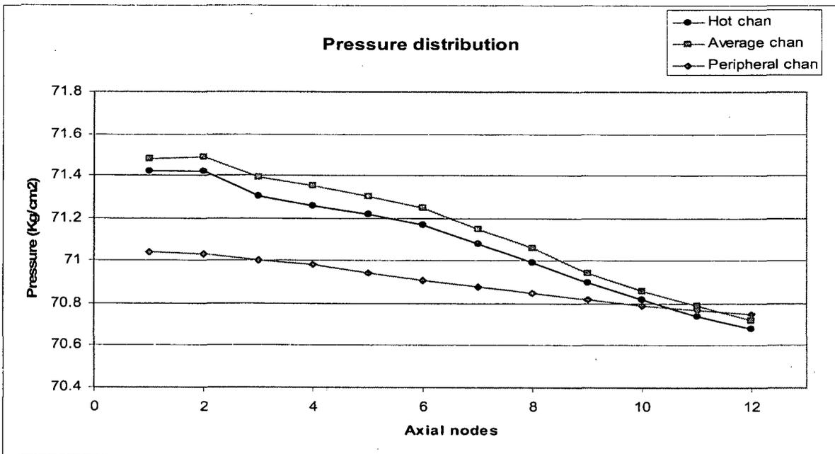
Figure 21 Axial pressure distribution
