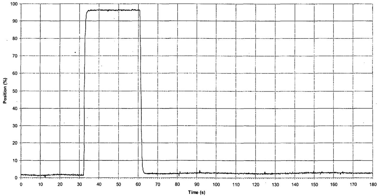
**Figure 11 Bypass valve position (plant data)**
