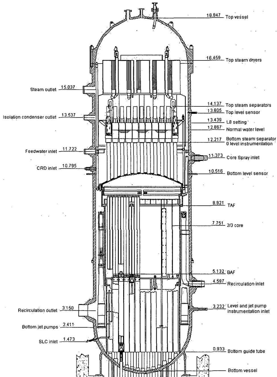
**Figure 13 Dimensions of the vessel geometry**
