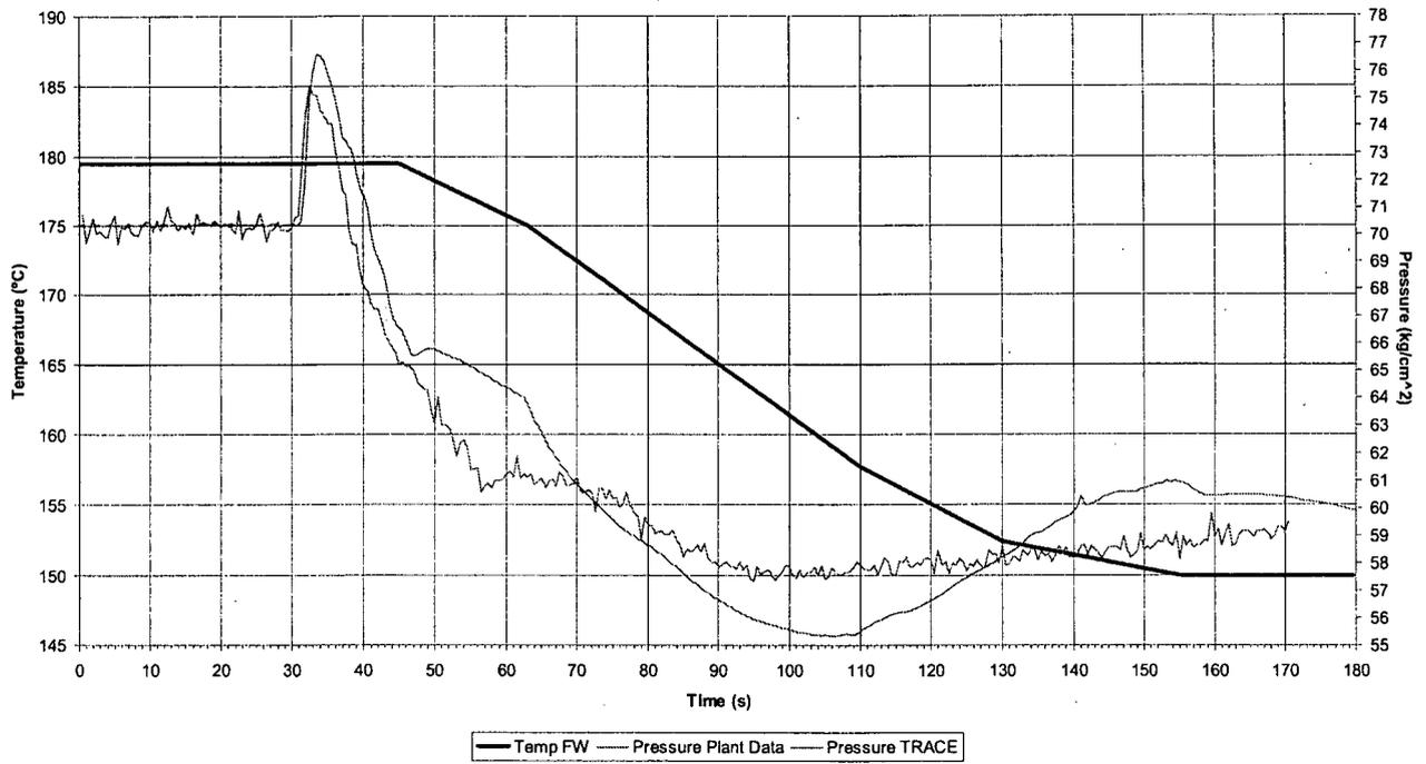
Figure 29 Feedwater temperature and reactor pressure (real and calculated)
