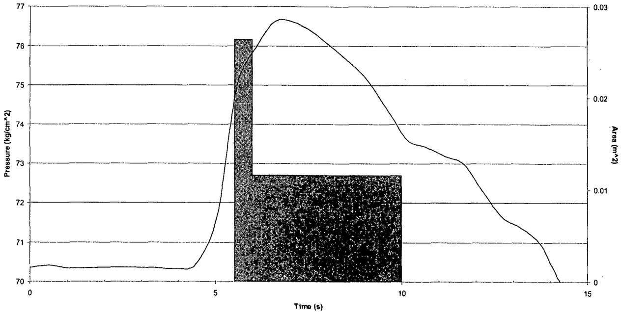
Figure 28 Combined graph of reactor pressure and area of RV/SRV
