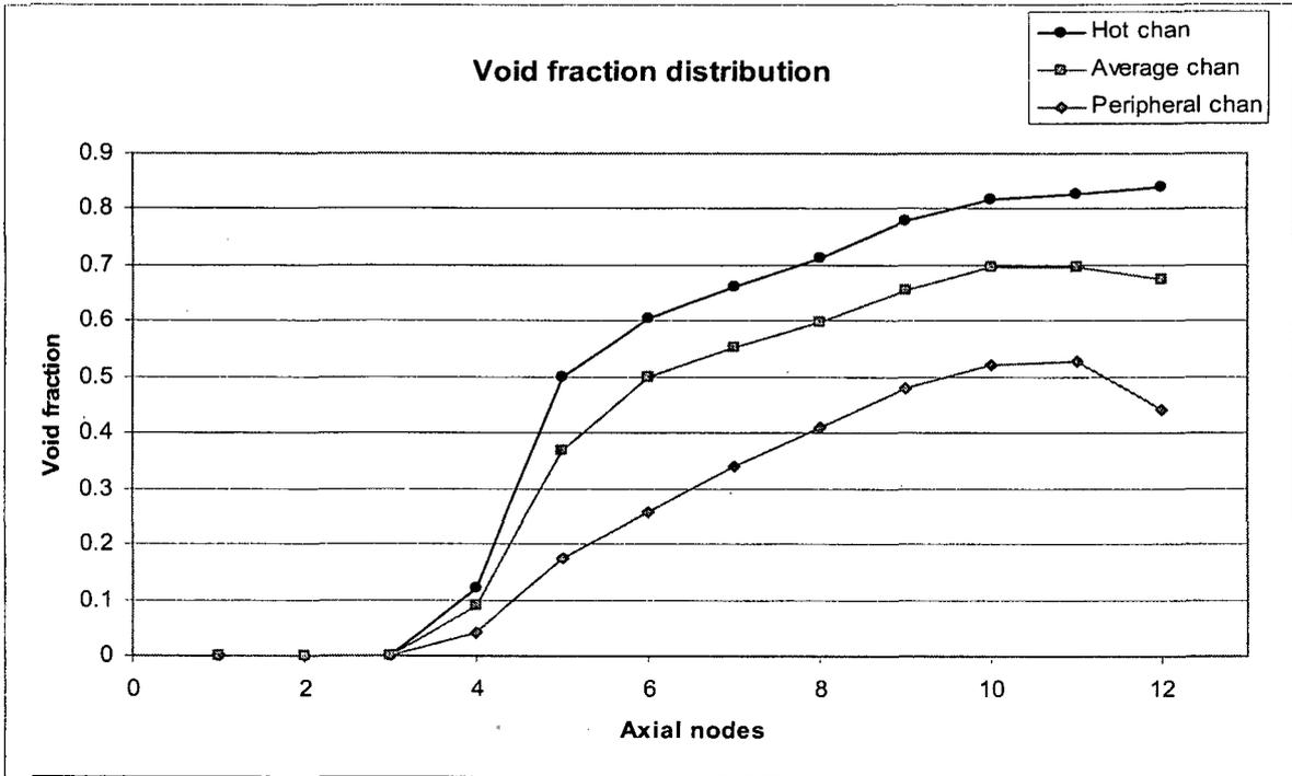
Figure 20 Axial void fraction distribution
