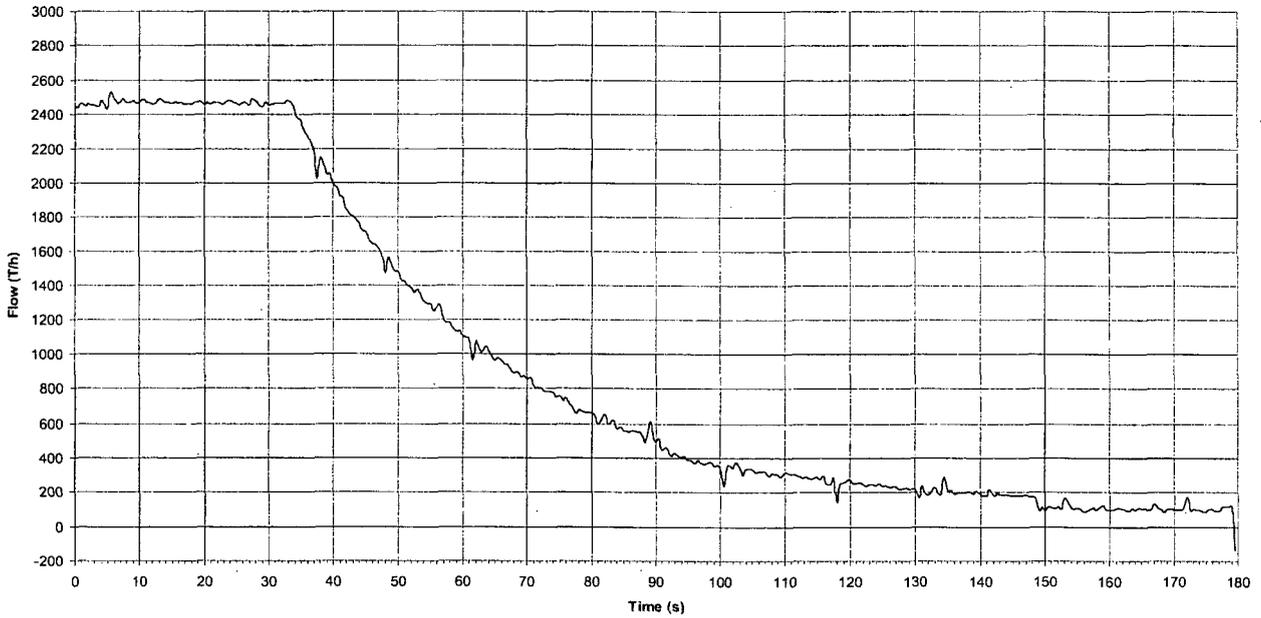
**Figure 5 Steam flow (plant data)**
