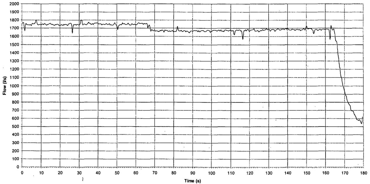
**Figure 9 Recirculation flow rate B (plant data)**
