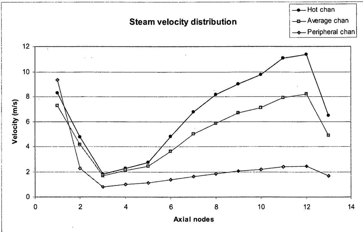
Figure 24 Axial steam velocity distribution
