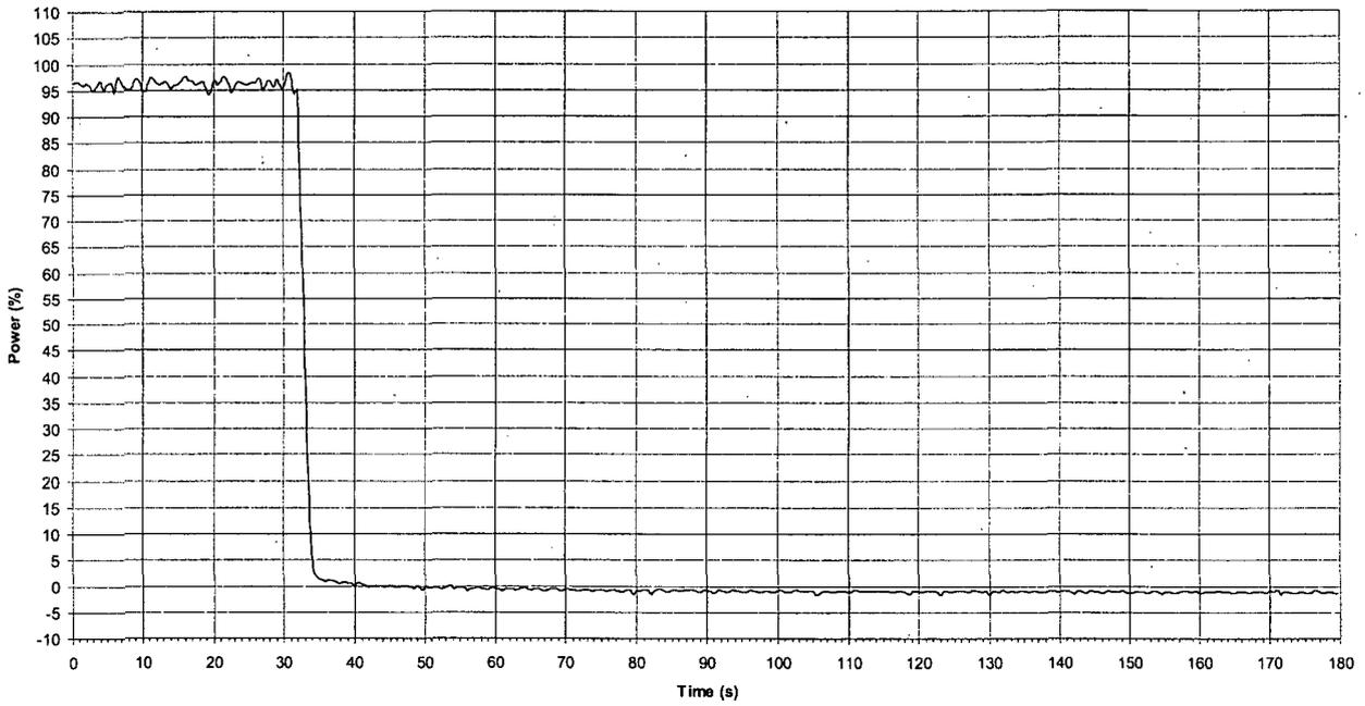
**Figure 2 Reactor power (plant data)**
