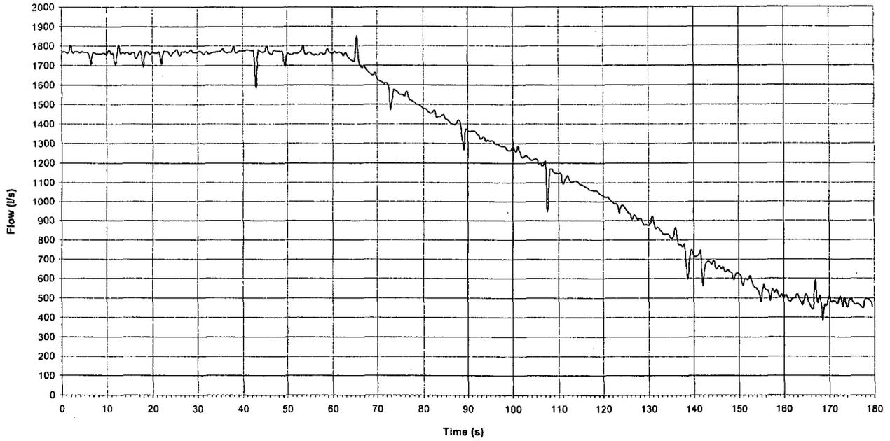
**Figure 8 Recirculation flow rate A (plant data)**
