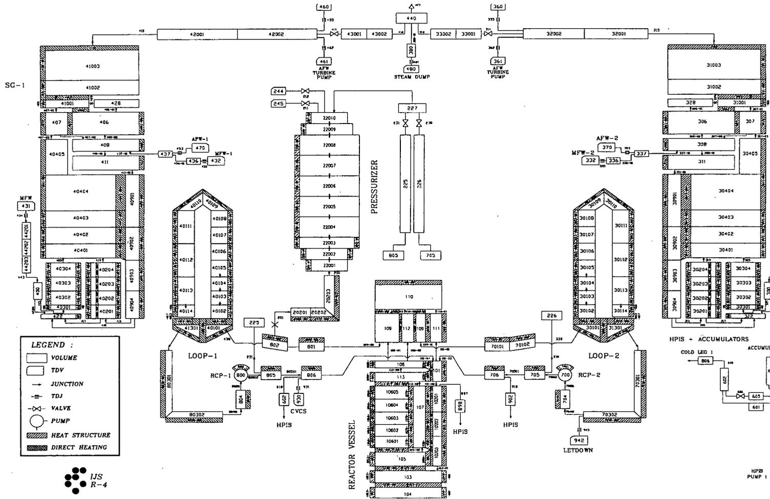
Figure 1 Krško NPP nodalization scheme
