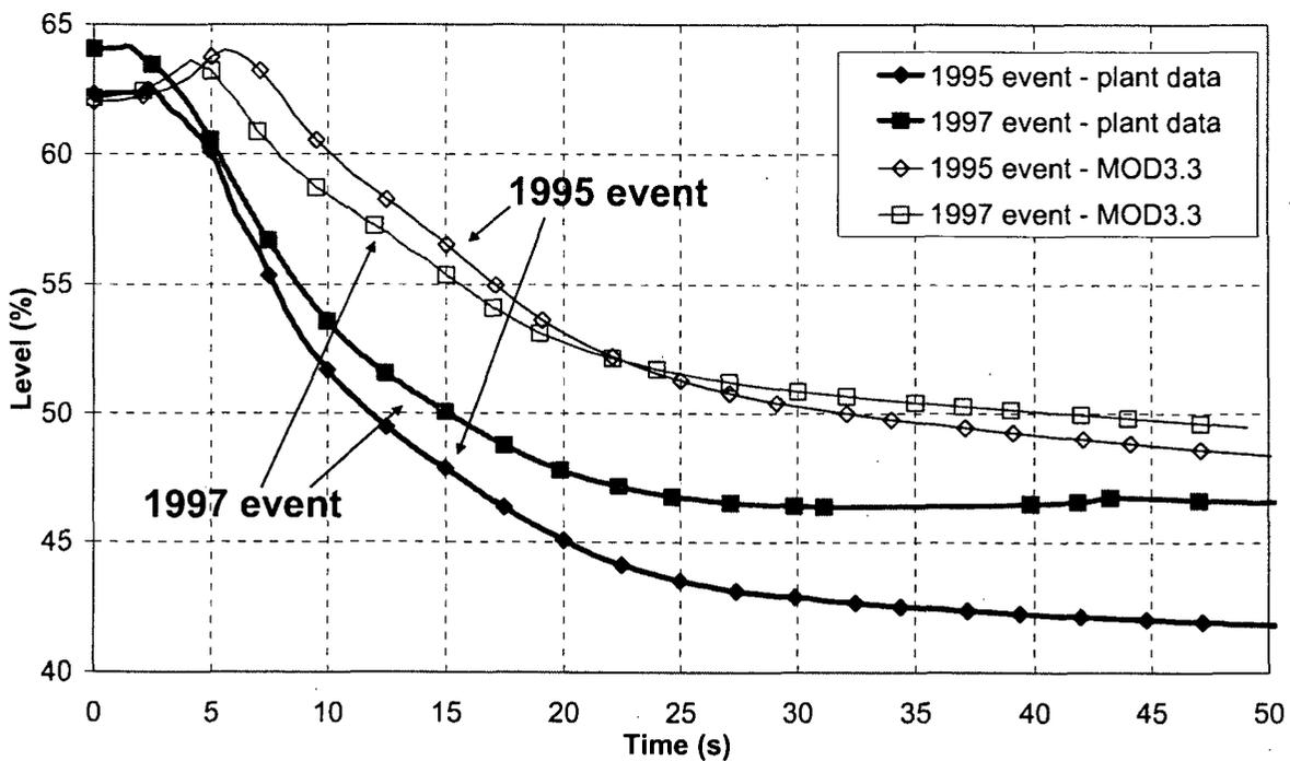
Figure 7 Pressurizer level
