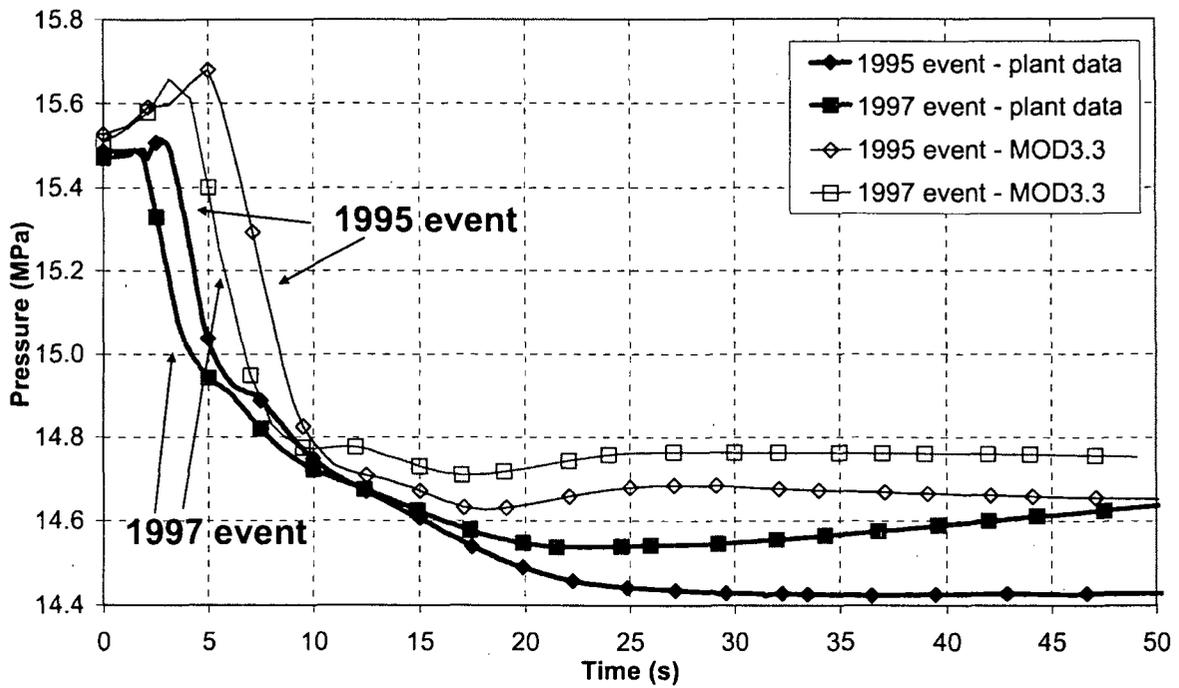
Figure 6 Pressurizer pressure
