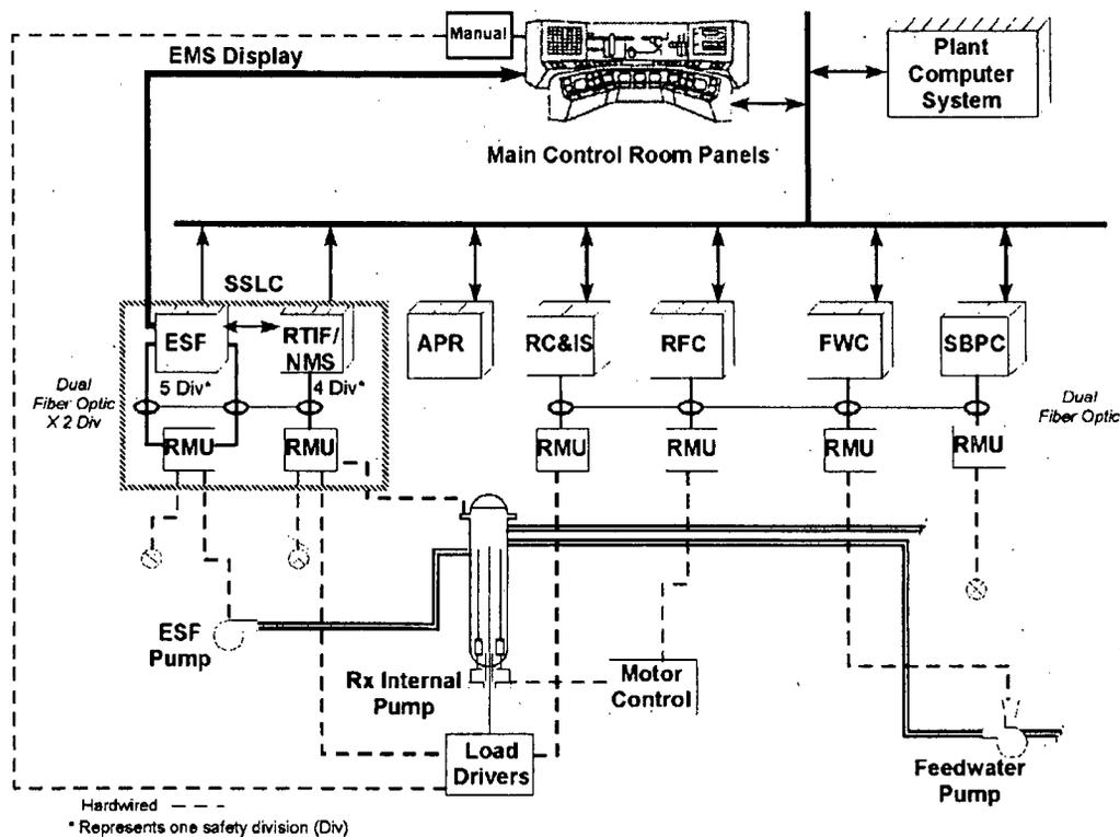
Fig. 4.10. Overall architecture of Lungmen I&C systems. (Adapted from Ref. 108.)
