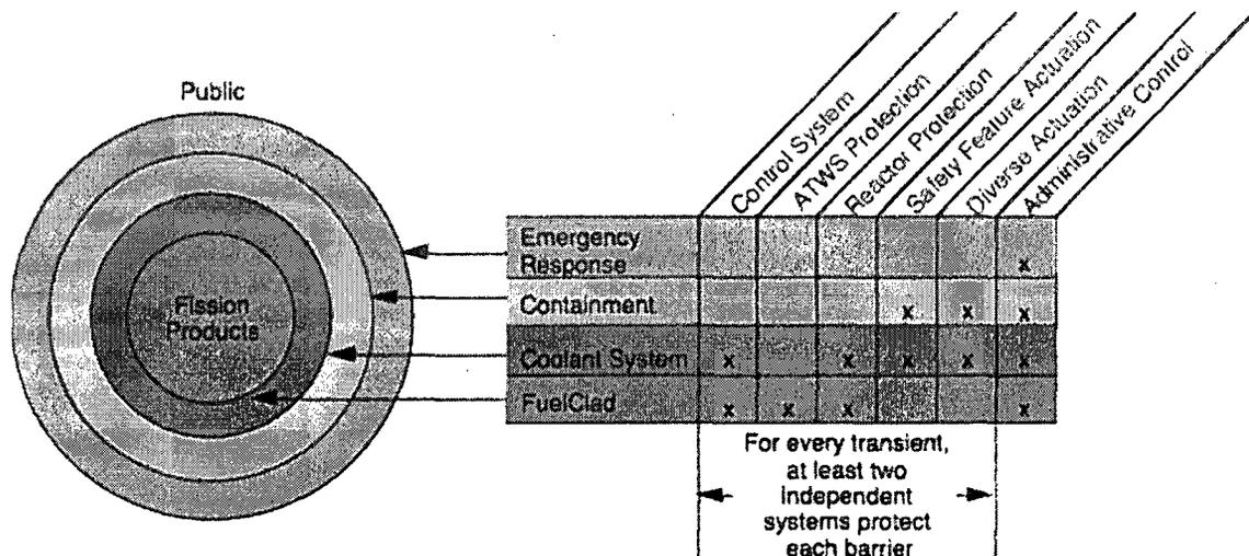
Fig. 2.2. Representation of I&C system architecture lines of defense.
