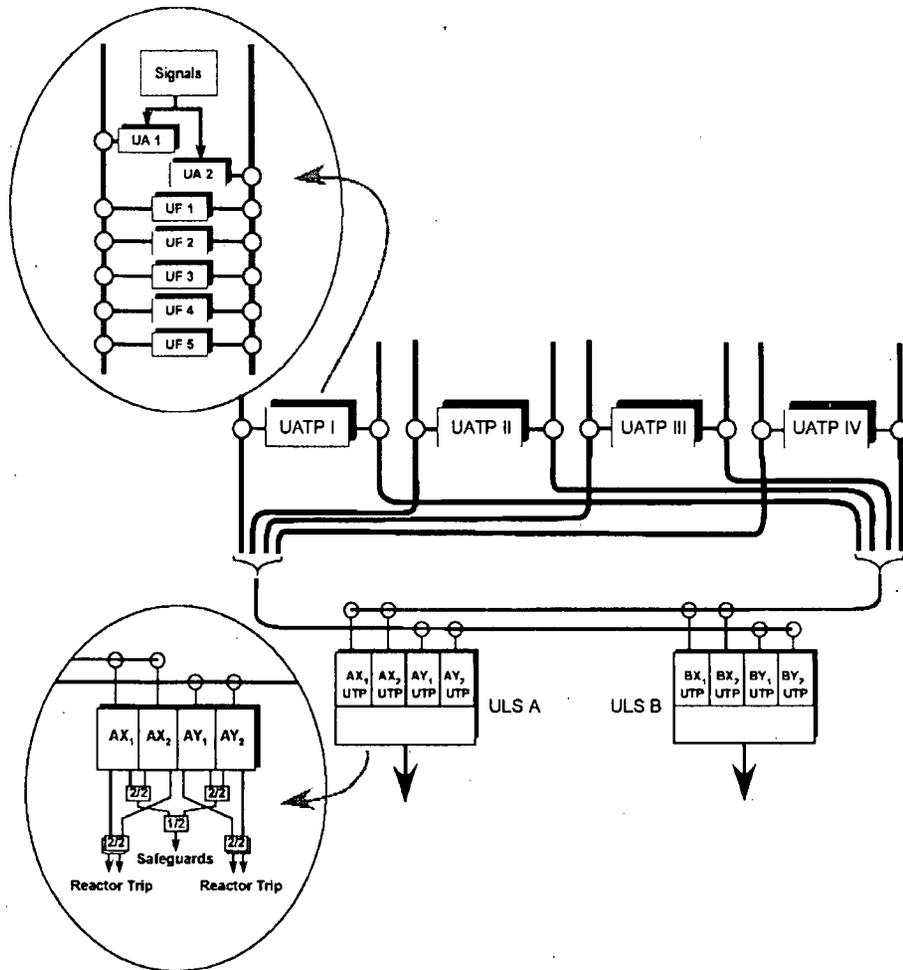
Fig. 4.6. SPIN architecture. (Adapted from Ref. 97.)
