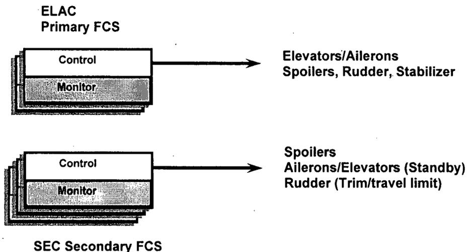
Fig. 3.2. Airbus A320 architecture. (Adapted from Ref. 44.)
