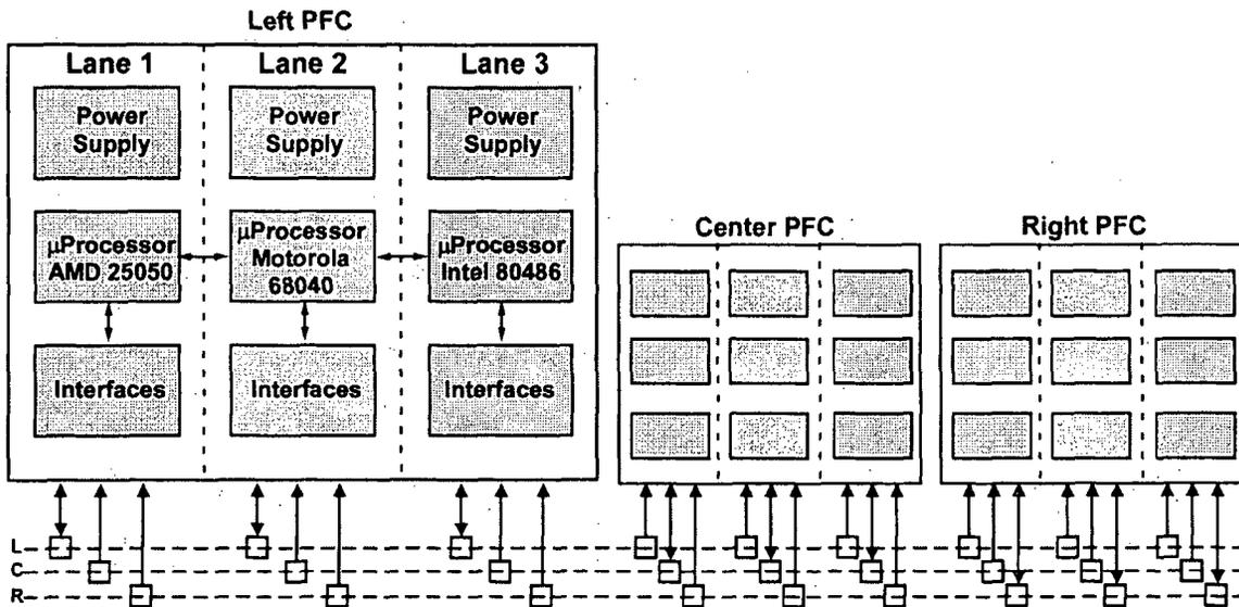
Fig. 3.3. Triple-triple redundancy architecture of the primary flight computer. (Adapted from Ref. 55.)
