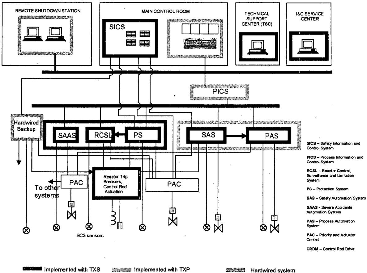
Fig. 4.11. Olkiluoto-3 I&C architecture. (Adapted from Ref. 110.)
