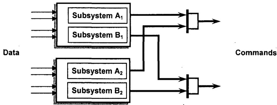
Fig. 4.3. Functionally diverse subsystems.
