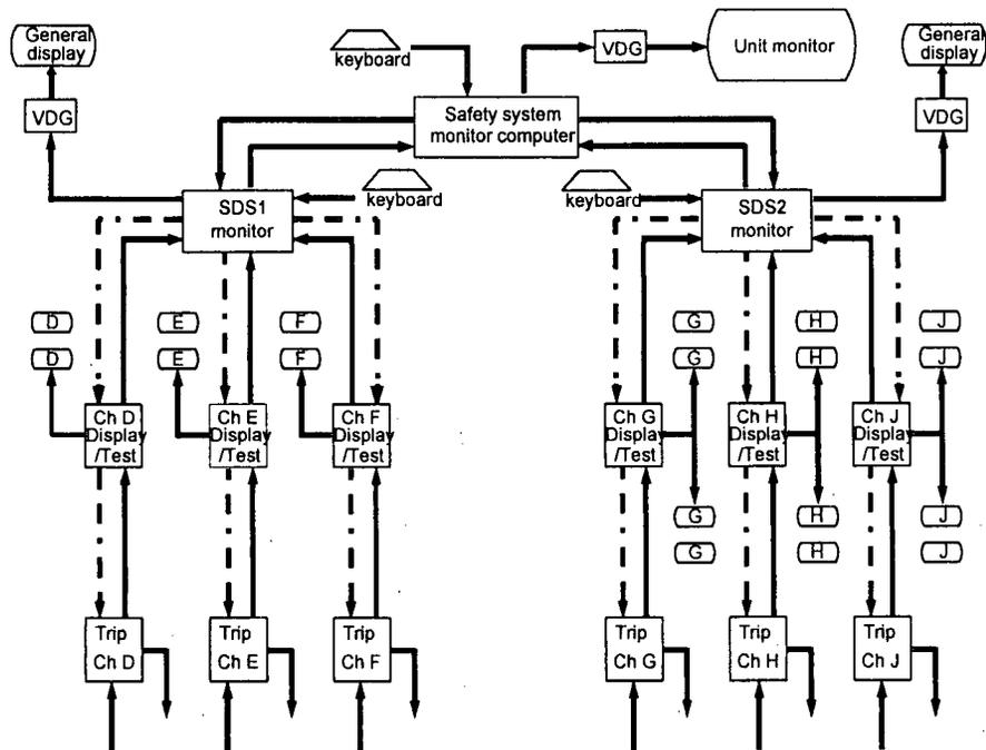
Fig. 4.4. Fully computerized shutdown system.
