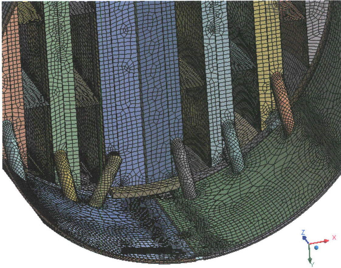
Figure 5c. Close up of mesh showing drain pipes and hood supports.
