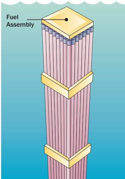
**2** After about 6 years, spent fuel assemblies—typically 14 feet (4.3 meters) long and containing nearly 200 fuel rods for PWRs and 80–100 fuel rods for BWRs—are removed from the reactor and allowed to cool in storage pools for a few years. At this point, the 900-pound (40.8 kilograms) assemblies contain only about one-fifth the original amount of uranium-235.
