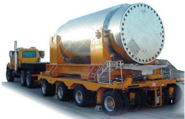
*Empty storage transport container on a semi tractor-trailer rig.*
