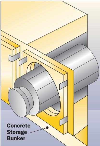
**2** The canisters can also be stored in aboveground concrete bunkers, each of which is about the size of a one-car garage.
