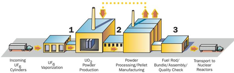
Fabrication is the final step in the process used to produce uranium fuel. Fuel fabrication facilities mechanically and chemically process the enriched uranium into nuclear reactor fuel.
