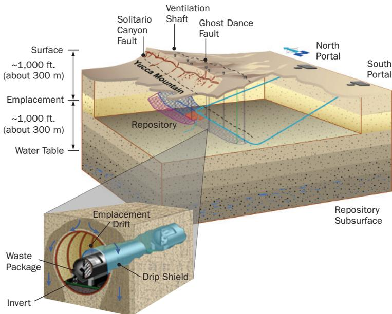
This cutaway image of Yucca Mountain details its planned network of repository surface facilities, ramps, tunnels, and cask emplacement.
