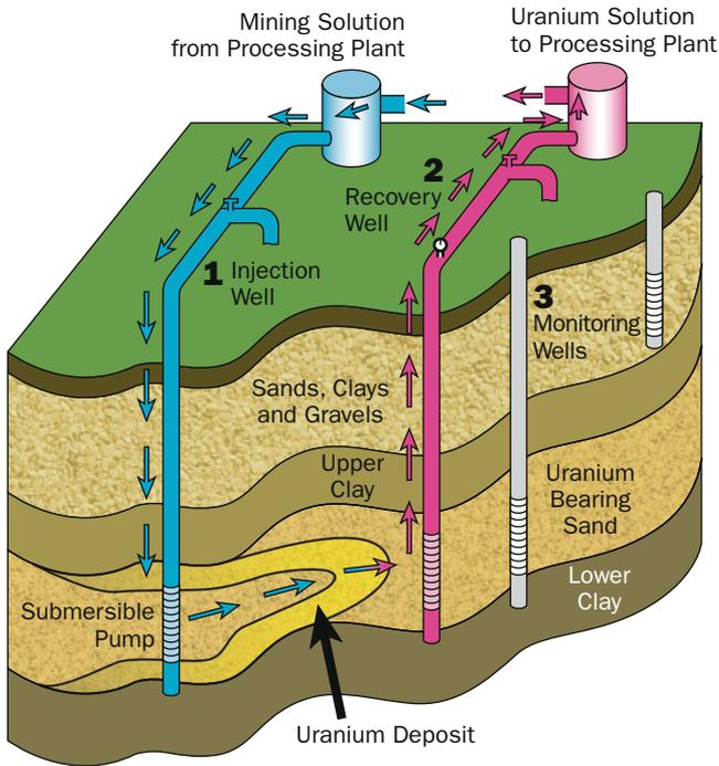
**Injection wells (1)** pump a chemical solution—typically sodium bicarbonate and oxygen—into the layer of earth containing uranium ore. The solution dissolves the uranium from the deposit in the ground and is then pumped back to the surface through **recovery wells (2)** and sent to the processing plant to be converted into uranium yellowcake. **Monitoring wells (3)** are checked regularly to ensure that uranium and chemicals are not escaping from the drilling area.
