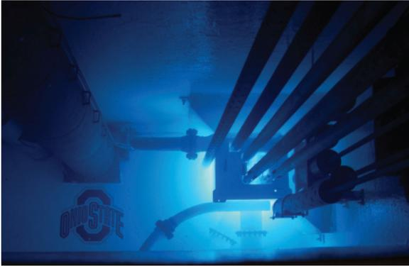
*A blue glow of radiation, known as the “Cerenkov effect,” from nuclear fuel in the Ohio State Research/Test Reactor*
