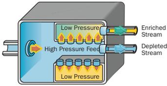
The gaseous diffusion process uses molecular diffusion to separate a gas from a two-gas mixture. The isotopic separation is accomplished by diffusing uranium, which has been combined with fluorine to form uranium hexafluoride ( $UF_6$ ) gas, through a porous membrane (barrier) and using the different molecular velocities of the two isotopes to achieve separation.
