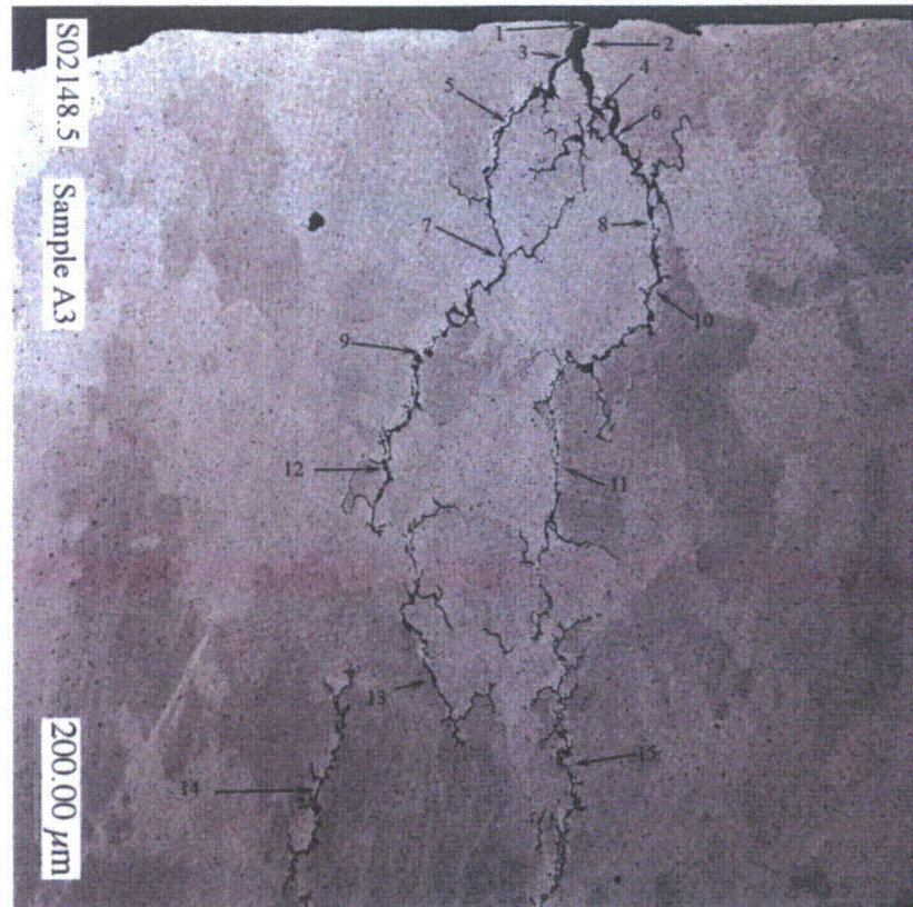
Figure 8.4 Crack CODs at Several Points Close to the Surface
