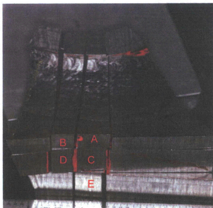
Figure 6.15 Cracked Metal Coupons Removed from Section 2
