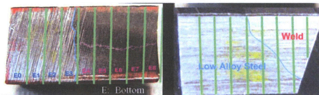
Figure 6.18 Bottom (left) and Side (right) Surfaces for E with Proposed Serial Sectioning. Note that these images are not to scale with those in Figure 6.17.
