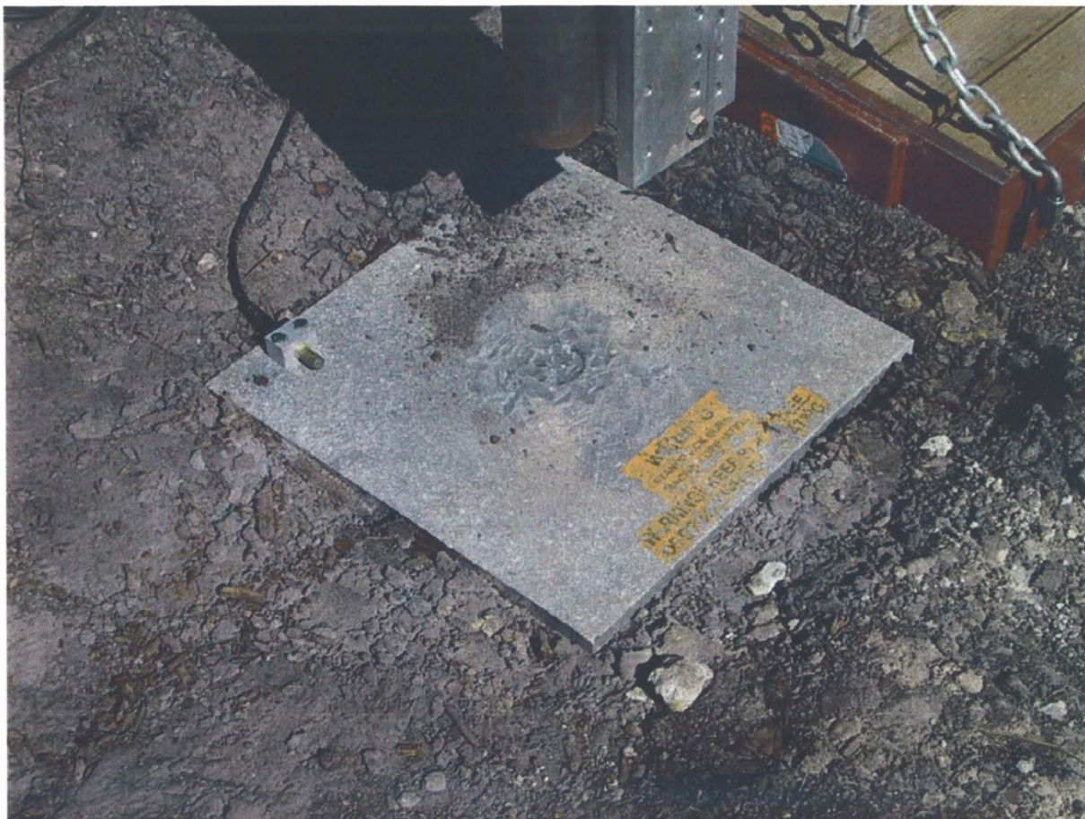
Figure 3: Downhole P-wave striking plate with hammer switch
