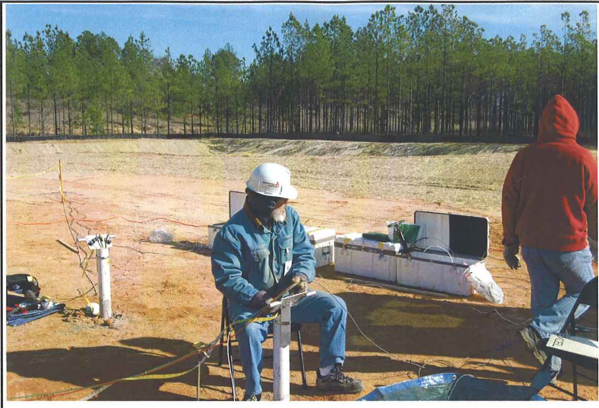
Photo 25. January 25, 2008 – Cross-Hole seismic triggering is being performed by Dr. Stokoe while others record the data.
