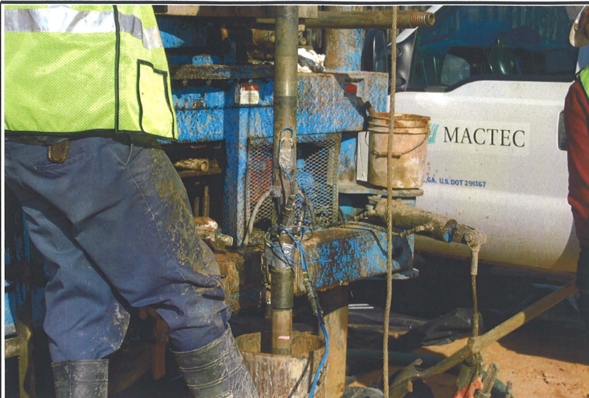
Photo 19. January 15, 2008 – SPT hammer energy calibration during drilling of boring drilled for Cross-Hole seismic testing.
