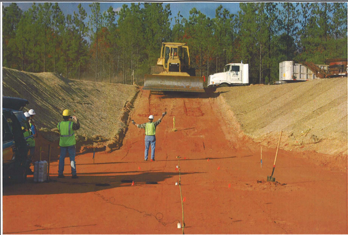
Photo 13. December 9, 2007 – Dr. Stokoe directs the bulldozer that is providing vibrations required for SASW testing, at depth.
