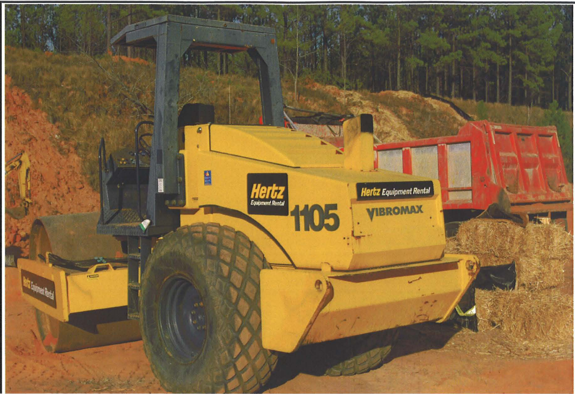
Photo 5. December 4, 2007- Vibromax 1105 vibratory smooth drum roller used to compact test pad fill.
