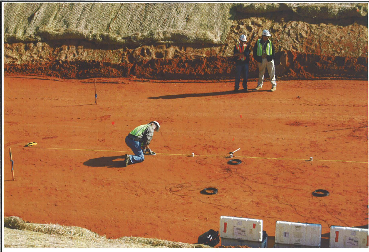
Photo 11. December 9, 2007- Dr. Stokoe generates vibrations for Spectral Analysis of Surface Wave (SASW) testing, at shallow depth.
