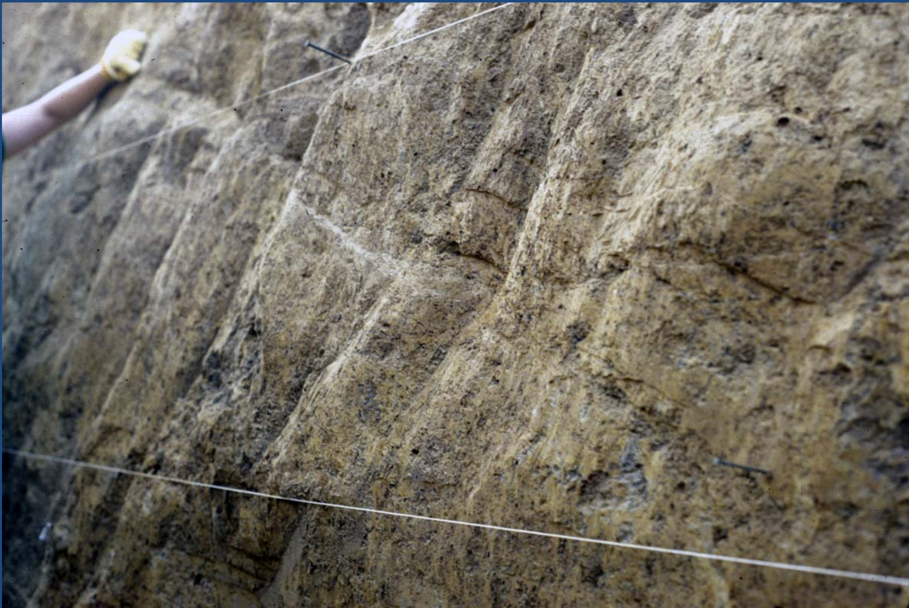
NE verging thrust fault in Kentucky River terrace colluvium.
