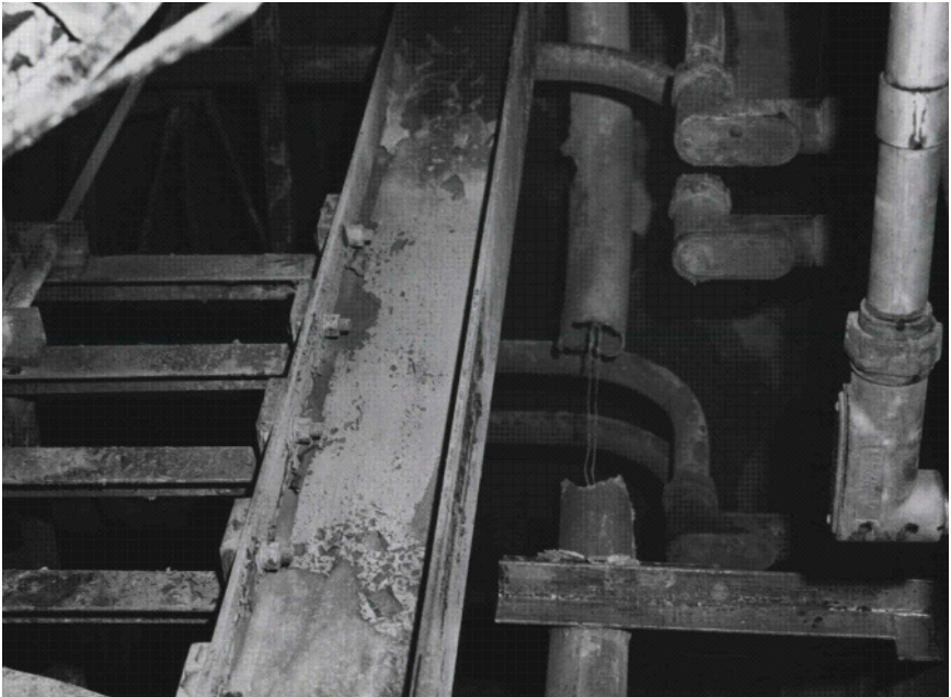
Picture of Browns Ferry Fire Cable Spreading Room. Note the melted aluminum electrical cable conduit. (TVA File Photo)
