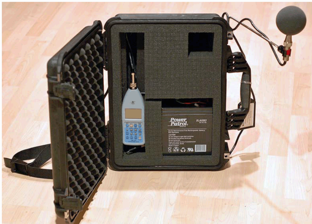
Figure 5.1.1: Data logger shown in weatherproof case with power supply and remote microphone.
