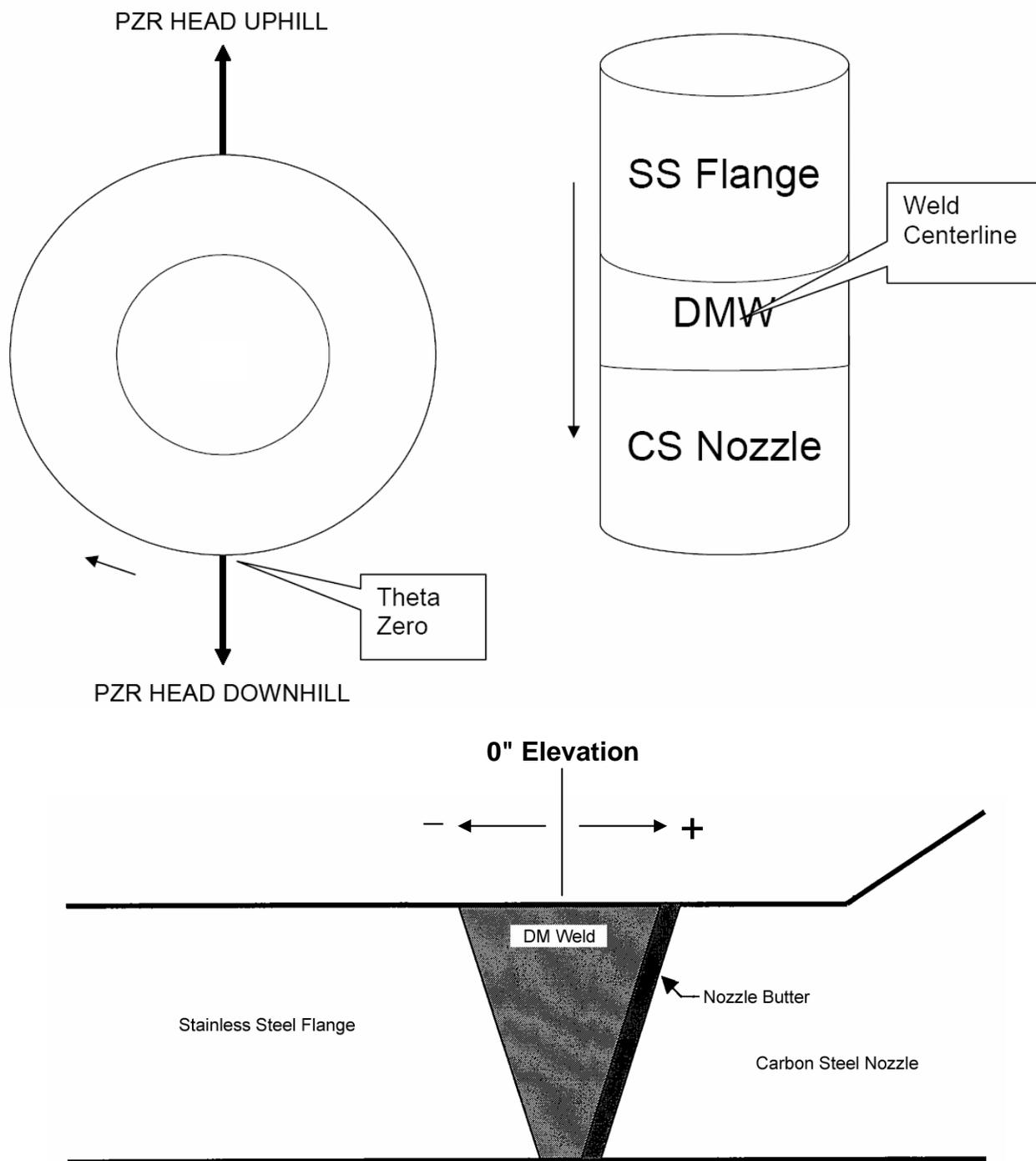
Figure 3: Orientation scheme and general configuration for nozzle/flange dissimilar metal weld. Degrees are increased in the clockwise direction when looking into head. The weld centerline was assigned the zero elevation, with elevation increasing when moving toward the head.
