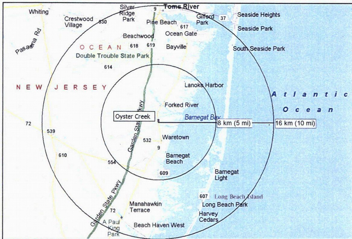
**Figure 6.1** - Approximation of the emergency planning zone for a nuclear power plant showing radial roadway networks.
