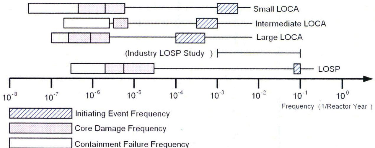
**Figure 3.5 -** Ranges of initiating event frequencies and corresponding core damage and containment failure frequencies for LOSP and LOCA based on NUREG-1150 site risk analysis reports for the Surry, Sequoyah, Grand Gulf and Peach Bottom reactors.
