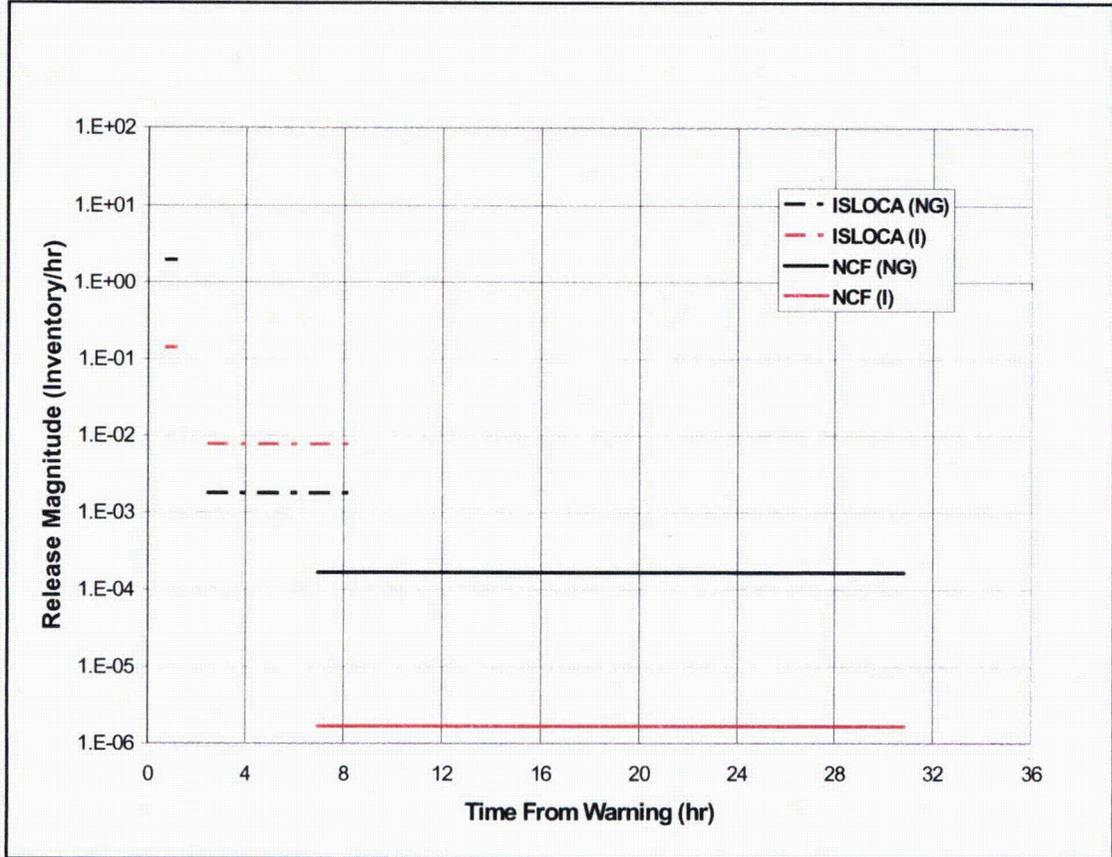
**Figure 5.3** - Comparison of the noble gas (NG) and halogen (I) release rates and durations for a typical Surry non-bypass no containment failure (NCF) and ISLOCA. The NCF source term is typical of major internal and external initiating events resulting in vessel breach and no vessel breach.
