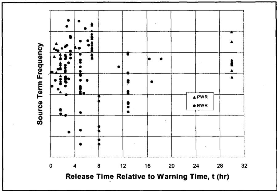
**Figure 3.1** - Release time corrected to warning time associated with site specific source terms for the Surry, Sequoyah, Grand Gulf, Peach Bottom, and LaSalle light water reactor sites due to internally and externally initiated events.
