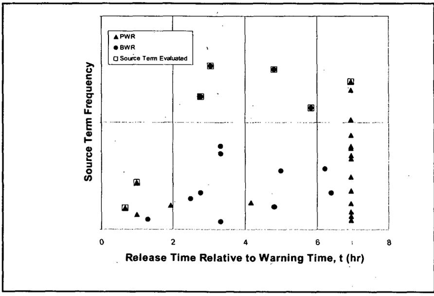
**Figure 3.2** - Higher frequency short time scale source terms for internally and externally initiated events at Surry, Sequoyah, Grand Gulf, Peach Bottom and LaSalle. Boxes indicate those source terms evaluated for potential use in the protective action recommendation study.
