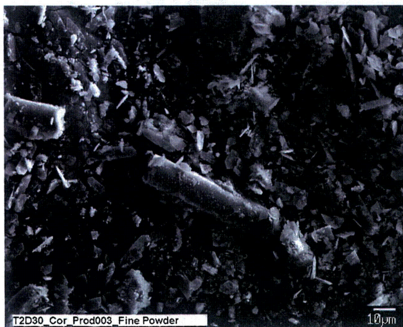
Figure B-4. Another SEM image at 650× magnification for a Test #2, Day-30 sample of fine powder on a vertical piece of the submerged PVC rack. The cylinder-shaped debris is likely to be fiberglass. (T2D30_Cor_Prod003_Fine Powder)
