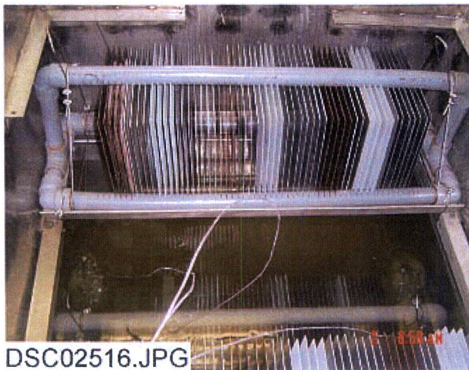
Figure 3-3. Loaded coupon rack in the ICET tank.
