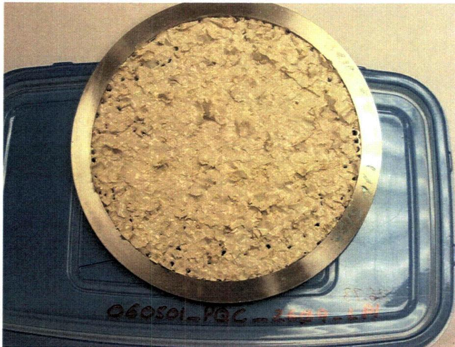
**Figure K.1.7. 060501\_PQC\_2609\_LP1, LP2 Debris Bed After Retrieval from Test Section, Top View**
