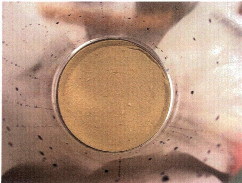
**Figure J.14.4. 051115\_NC\_4098\_L1 Debris Bed in Test Section After Retrieval, Top View. Apparent gap from debris bed to test-section wall and collapsed rim at the 2:00 position were caused after test section retrieval from test loop and prior to measurements being taken.**
