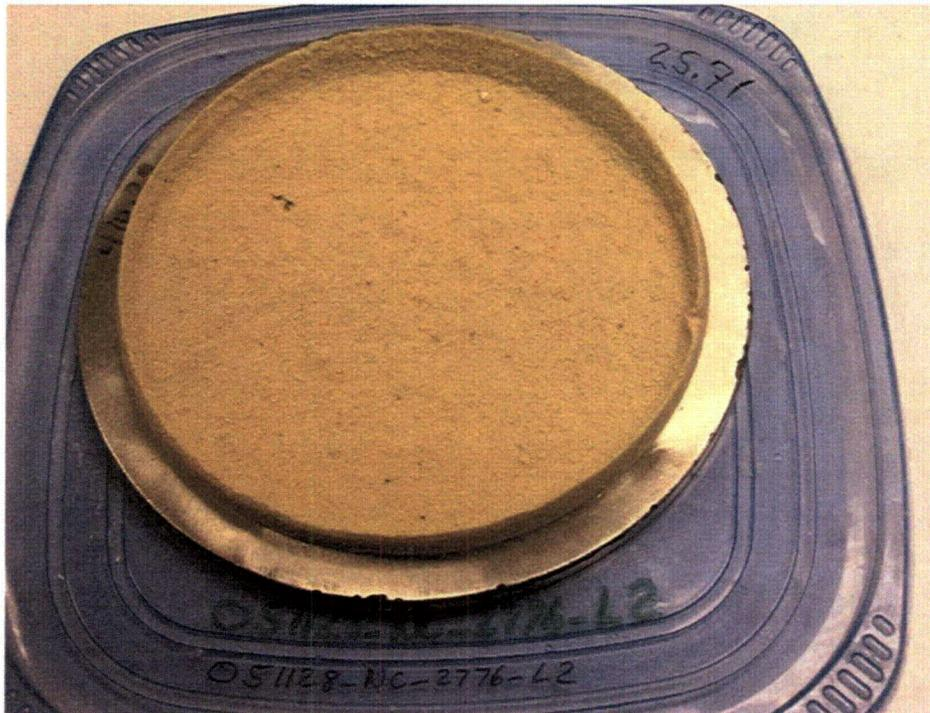
Figure J.13.6. 051128\_NC\_2776\_L2 Debris Bed After Retrieval from Test Section. Indentation on Debris Bed Rim at 3:15 Orientation Due to Post-Retrieval Handling.
