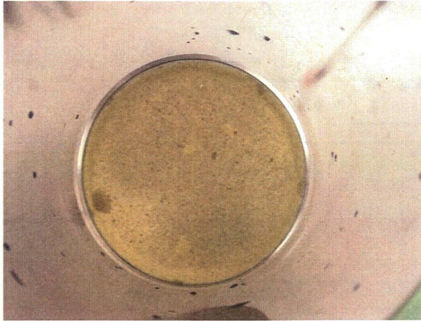
**Figure H.2.2. 060313\_NO\_1349\_LP1 Debris Bed in Test Section After Retrieval, Top View**
