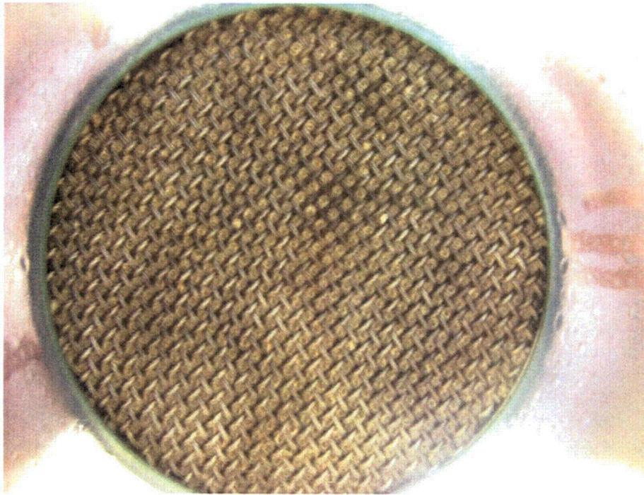
**Figure H.4.5. 051108\_NO\_3067\_L1 Debris Bed in Test Section After Retrieval, Bottom View**
