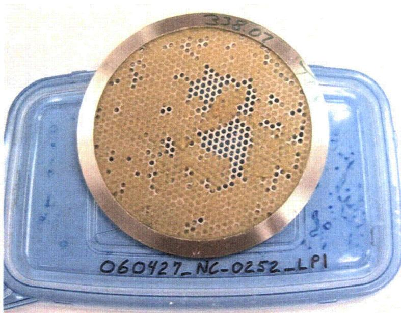
**Figure 7.33. Incomplete Debris Bed Retrieved from Test NC1 with a Retrieved Mass Loading of  $56.3 \text{ g/m}^2$ . The target mass loading was  $108 \text{ g/m}^2$  NUKON,  $27 \text{ g/m}^2$  CalSil, and  $135 \text{ g/m}^2$  total.**
