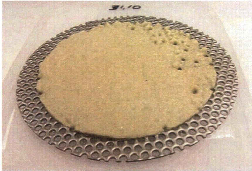
**Figure 7.24. Incomplete Debris Bed from COBT6, Test 060510\_CO\_2351\_BP3. Target CalSil mass loading = 2900 g/m<sup>2</sup>, retrieved CalSil mass loading = 390 g/m<sup>2</sup>, 13% of target mass retained on screen, debris bed formed in the benchtop test loop.**
