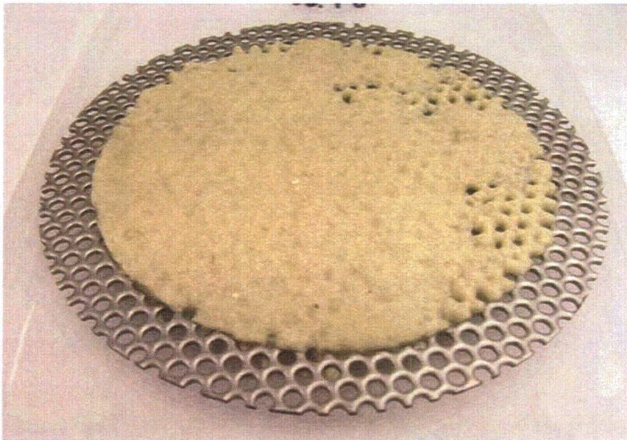
**Figure 7.22. Incomplete Debris Bed from COBT2, Test 060510\_CO\_1469\_BP1. Target CalSil mass loading = 1812 g/m<sup>2</sup>, retrieved CalSil mass loading = 237 g/m<sup>2</sup>, 13% of target mass retained on screen, debris bed formed in benchtop test loop.**
