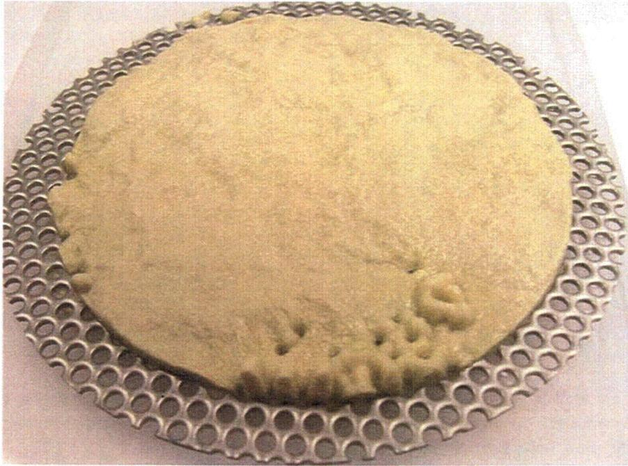
**Figure 7.25. Incomplete Debris Bed from COBT7, Test 060511\_CO\_3527\_BP2. Target CalSil mass loading = 4350 g/m<sup>2</sup>, retrieved CalSil mass loading = 724 g/m<sup>2</sup>, 17% of target mass retained on screen, debris bed formed in the benchtop test loop.**
