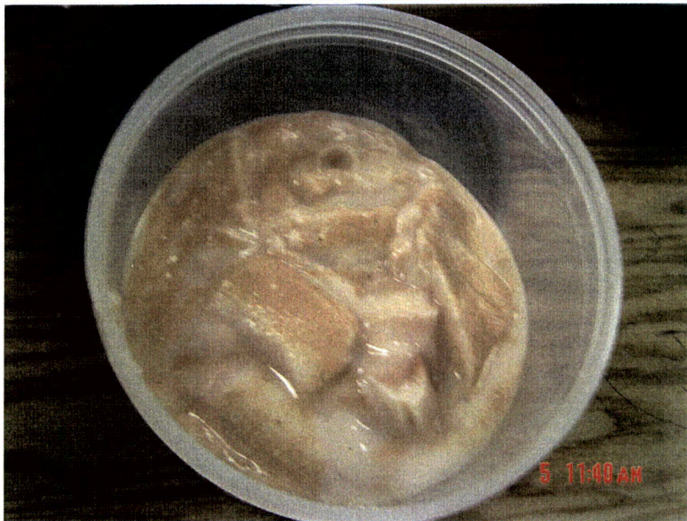
Figure 4-185. Gel-like material recovered from the bottom of the tank.
