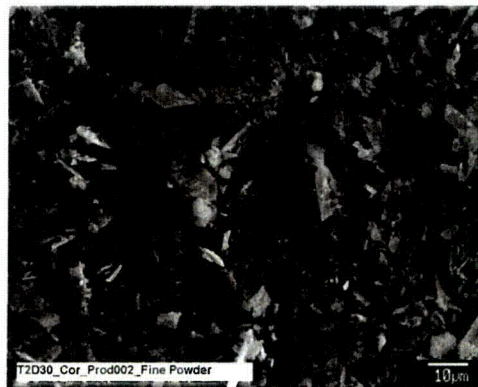
Figure 4-173. SEM image at 1000× magnification of a Test #2, Day 30, sample of fine powder on a vertical piece of the submerged PVC rack. (T2D30_Cor_Prod002_Fine Powder)
