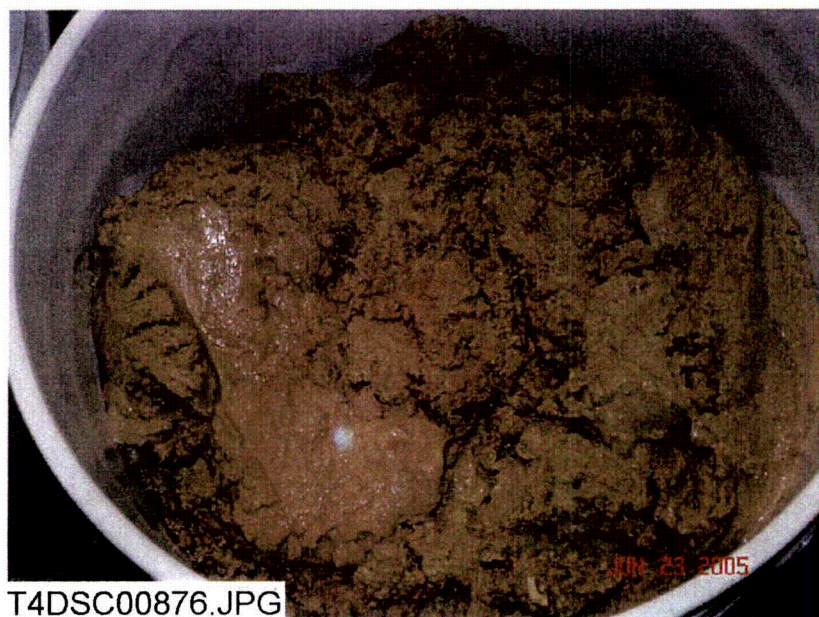
Figure 4-90. Sediment removed from the tank after Test #4.
