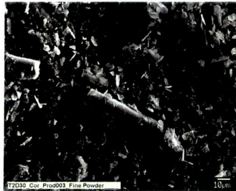
Figure 4-172. SEM image at 650× magnification of a Test #2, Day 30, sample of fine powder on a vertical piece of the submerged PVC rack. (T2D30_Cor_Prod003_Fine Powder)
