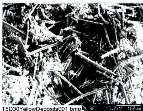
Figure 4-181. SEM image, magnified 100 times, of the Test #5 Day 30, fine yellow powder on the submerged rack. (T5D30YellowDeposits001.bmp)
