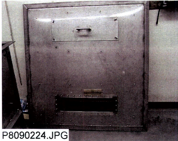
Figure A-8. The cover lid of the ICET tank showing the top observation window (lower) and top access hatch with handle (upper).
