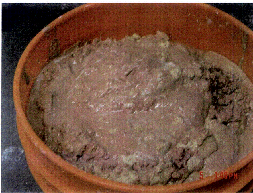
Figure 4-84. Sediment removed from the tank after Test #3.
