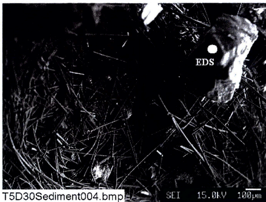
Figure 4-96. SEM image, magnified 70 times, of the Test #5, Day 30, sediment at the bottom of the tank.
