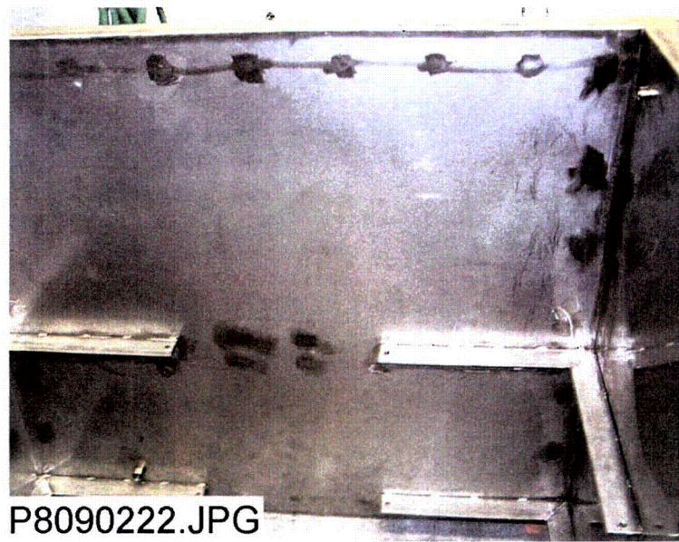
Figure A-6. The top and bottom angle irons for supporting coupon racks in the upper section of the ICET tank.
