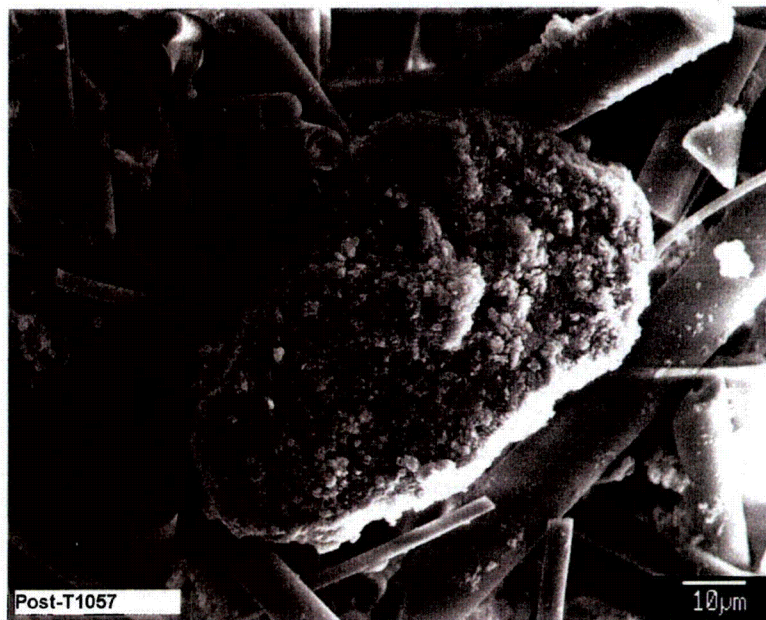
Figure 4-77. SEM image, magnified 1000 times, of a Test #1, Day 30, sediment sample.
