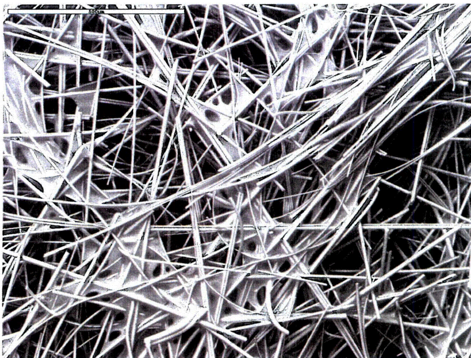
Figure 4-27. ESEM image, magnified 100 times, of raw fiberglass dipped in the solution containing 2800 mg/L boron and NaOH at pH 9.5. (Bofbrg09.tif, 8/3/05)
