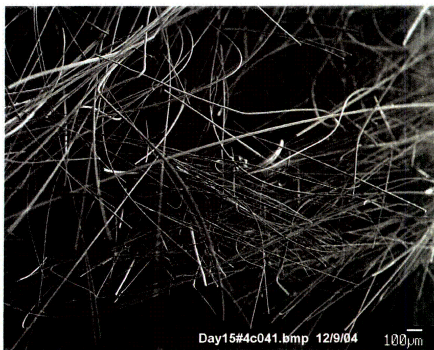
Figure 4-17. Clean fiberglass before exposure to test chemicals.
