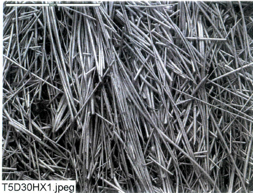
Figure 4-53. ESEM image, magnified 100 times, of a Test #5, Day 30, high-flow exterior fiberglass sample. (T5D30HX1.jpeg)
