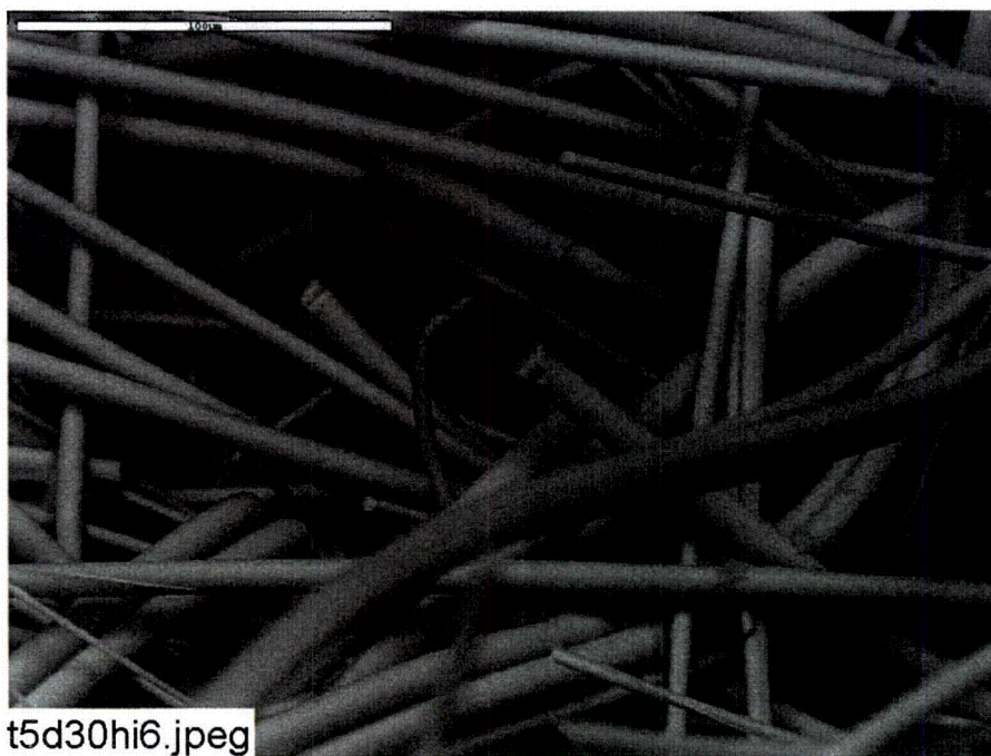
Figure 4-56. ESEM image, magnified 500 times, of a Test #5, Day 30, high-flow interior fiberglass sample. (t5d30hi6.jpg)
