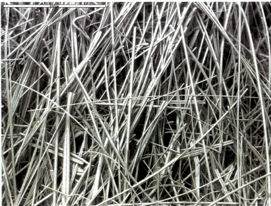
Figure 4-26. ESEM image, magnified 100 times, of raw fiberglass dipped in NaOH solution at pH 9.5. (OHFbrg07.tif, 8/3/05)
