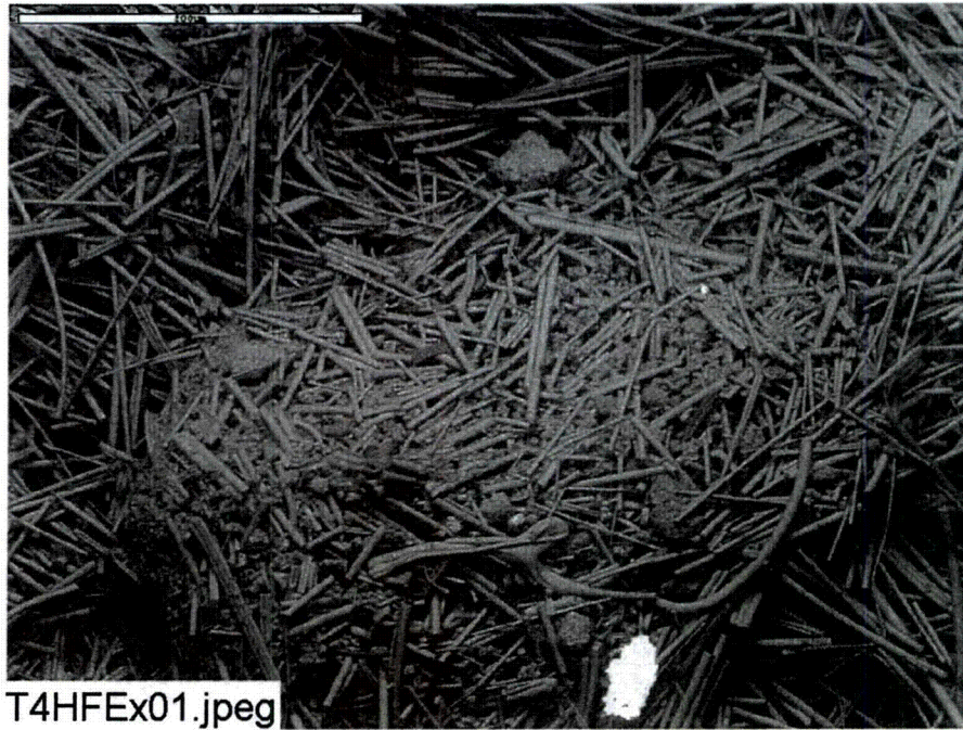
Figure 4-44. ESEM image, magnified 100 times, of a Test #4, Day 30, exterior high-flow fiberglass sample. (T4HFEx01.jpg)
