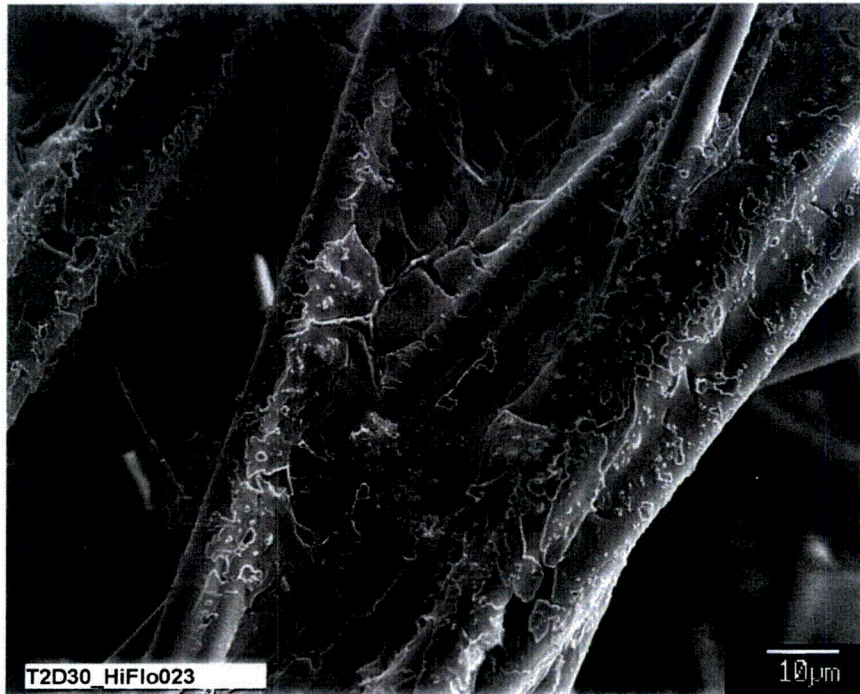
Figure 4-34. Probe SEM image at 1000× magnification for a Test #2, Day 30, high-flow interior fiberglass sample. (T2D30_HiFlo023)
