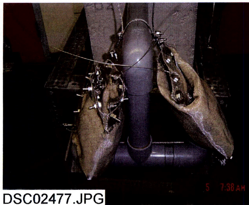
Figure 2-4. Fiberglass samples attached to a coupon rack.
