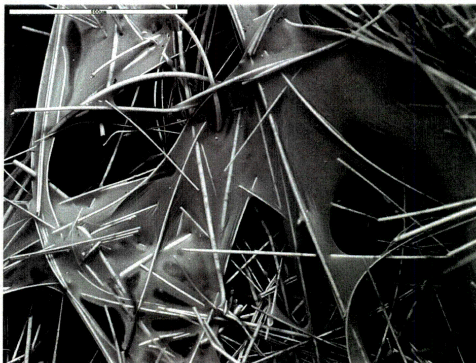
Figure 4-23. ESEM image, magnified 100 times, of raw fiberglass dipped in ICET Test #1 solution. (rfbt105.tif, 7/28/05)
