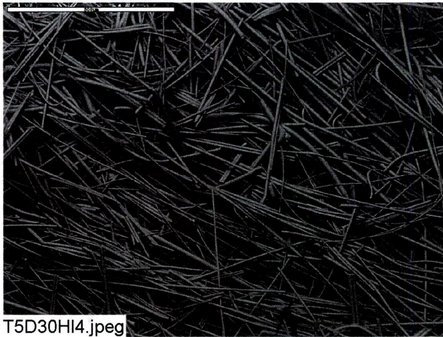
Figure 4-55. ESEM image, magnified 100 times, of a Test #5, Day 30, high-flow interior fiberglass sample. (T5D30HI4.jpg)
