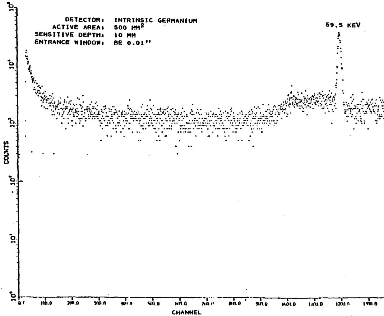
Figure B.2. Gamma-Ray Spectrum of ICSD Containing 3  $\mu$ Ci Am-241 Source.
