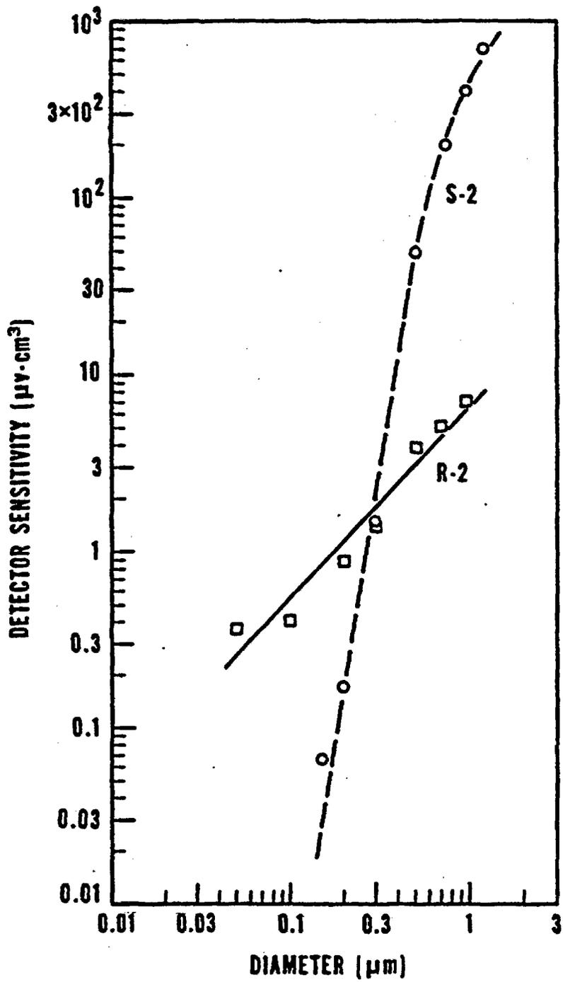
Figure 4.2. Detector Sensitivity Versus Particle Size for a Light-Scattering Type Detector (S-2) and for an Ionization Type Detector (R-2) <sup>2</sup>
