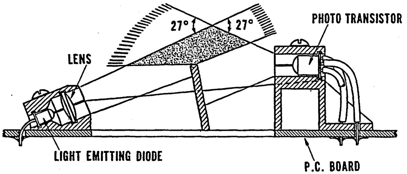
Figure 4.1. Photoelectric Detector Optics.<sup>2</sup>
