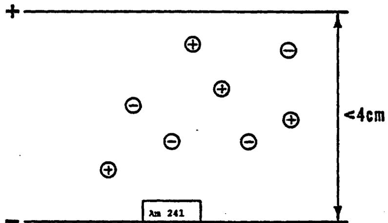
Figure 2.1. Bipolar Ionization Chamber<sup>2</sup>.
