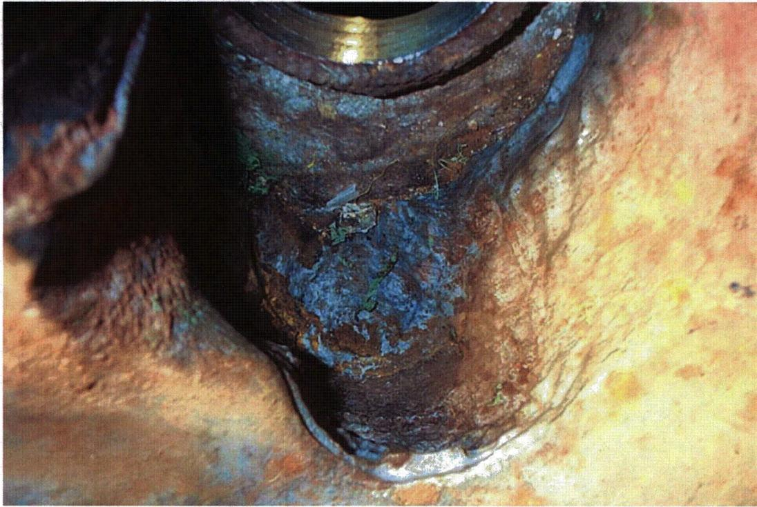
Figure B.18.6 Cavity in RPV head at D-B after removal of CRDM nozzle #3
