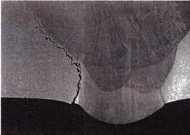
**Figure S.2** Intergranular stress corrosion cracking adjacent to a weld in 28" BWR recirculation pipe as has been observed in many BWR reactor coolant systems.
