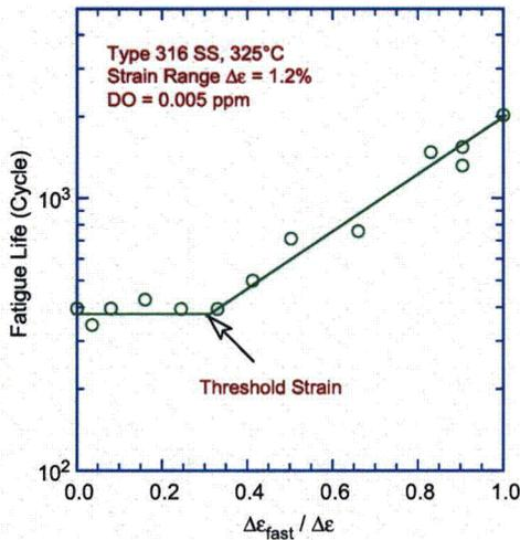
Figure 42. Results of strain rate change tests on Type 316 SS in low-DO water at 325°C. Low strain rate was applied during only a fraction of tensile loading cycle. Fatigue life is plotted as a function of fraction of strain at high strain rate (Refs. 24,29).
