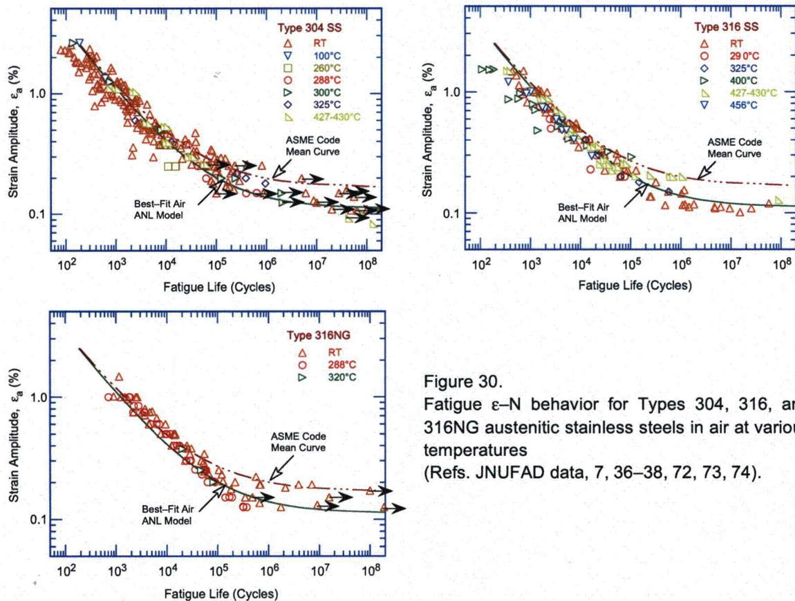
Figure 30. Fatigue  $\epsilon$ - $N$  behavior for Types 304, 316, and 316NG austenitic stainless steels in air at various temperatures (Refs. JNUFAD data, 7, 36-38, 72, 73, 74).
