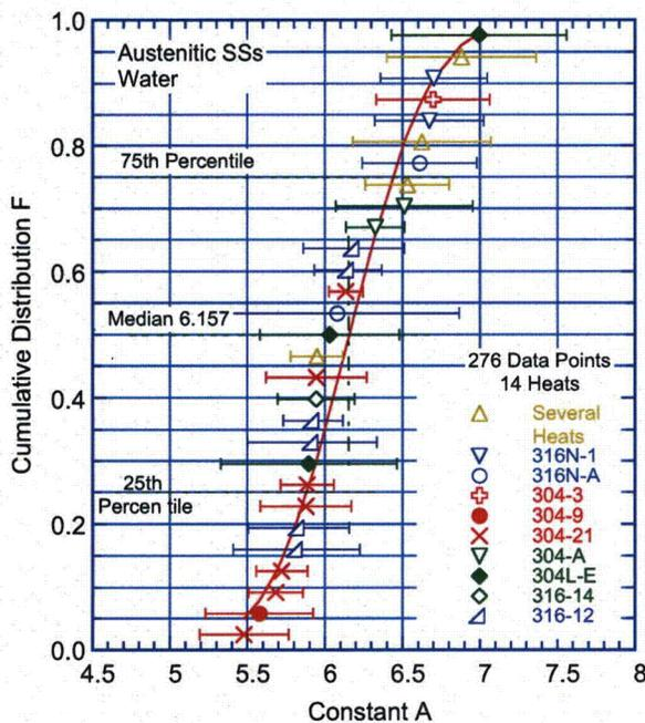
Figure 52. Estimated cumulative distribution of constant A in the ANL model for fatigue life for heats of austenitic SSs in water.
