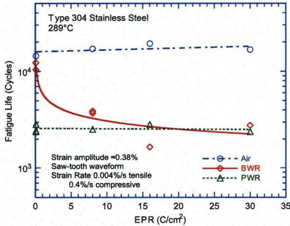
Figure 49. The effect of material heat treatment on fatigue life of Type 304 stainless steel in air, BWR and PWR environments at 289°C,  $\approx 0.38\%$  strain amplitude, sawtooth waveform, and 0.004%/s tensile strain rate (Ref. 40).
