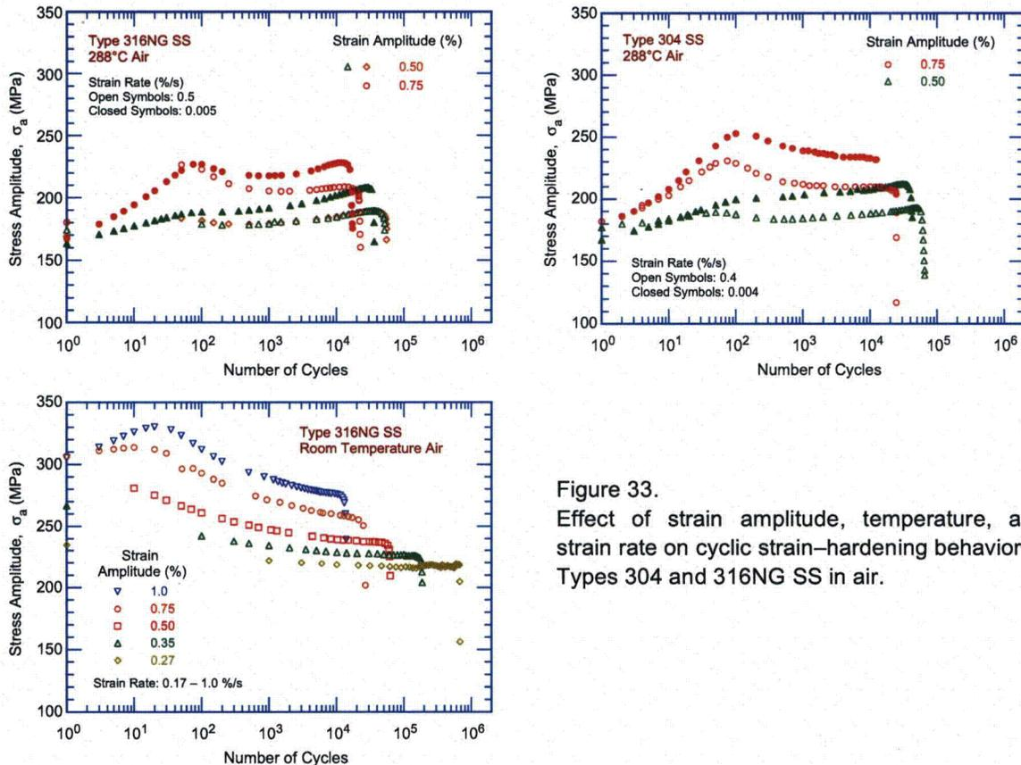
Figure 33. Effect of strain amplitude, temperature, and strain rate on cyclic strain-hardening behavior of Types 304 and 316NG SS in air.
