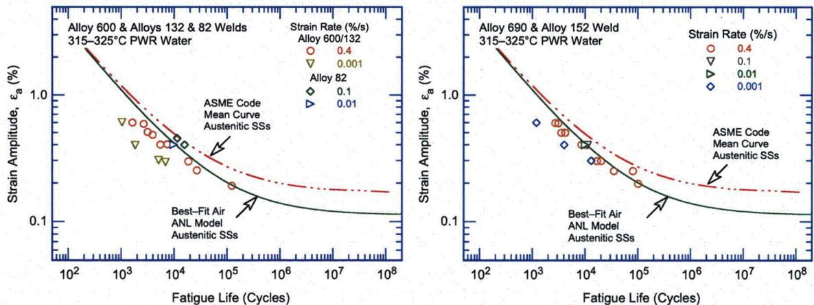
Figure 59. Fatigue  $\epsilon$ -N behavior for Alloys 600 and 690 and their weld alloys in simulated PWR water at  $315\text{--}325^\circ\text{C}$  (Refs. 33, 78).
