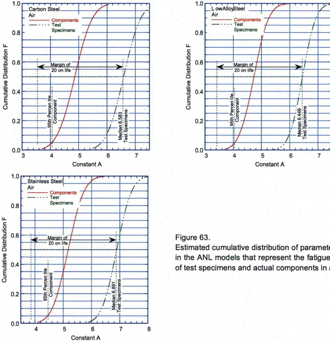
Figure 63. Estimated cumulative distribution of parameter A in the ANL models that represent the fatigue life of test specimens and actual components in air.
