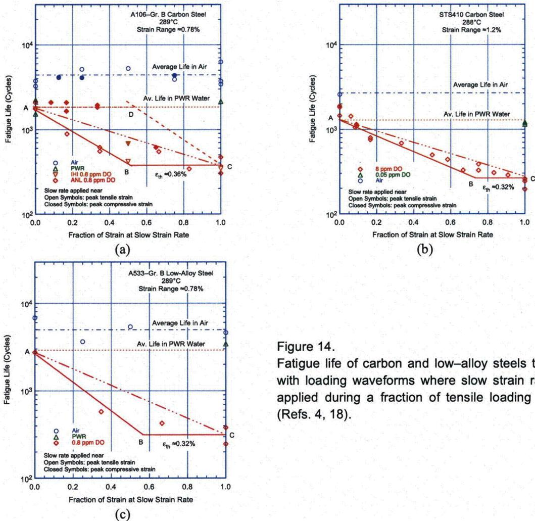
Figure 14. Fatigue life of carbon and low-alloy steels tested with loading waveforms where slow strain rate is applied during a fraction of tensile loading cycle (Refs. 4, 18).
