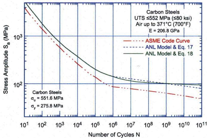
Figure 9. Fatigue design curve for carbon steels in air. The curve developed from the ANL model is based on factors of 12 on life and 2 on stress.
