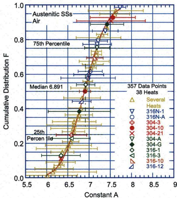
Figure 35. Estimated cumulative distribution of constant A in the ANL model for fatigue life for heats of austenitic SS in air.
