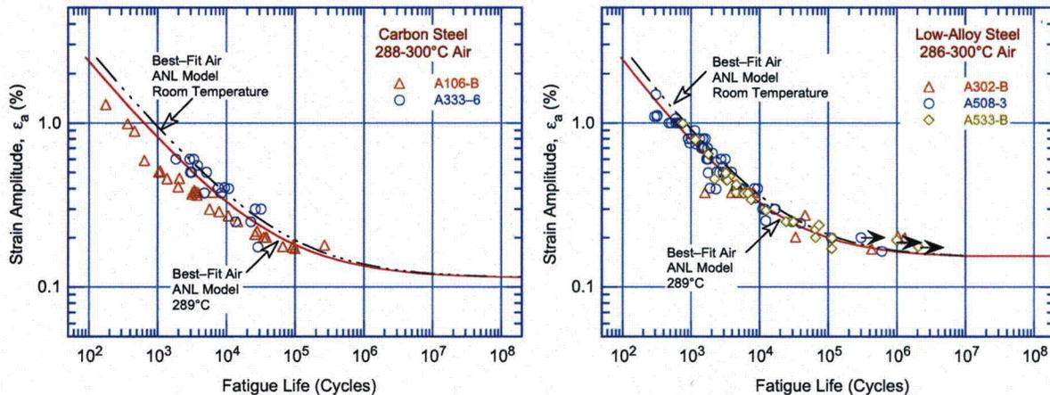
Figure 4. Fatigue strain vs. life data for carbon and low-alloy steels in air at 288°C (JNUFAD database, and Refs. 4,12,13,42,43).
