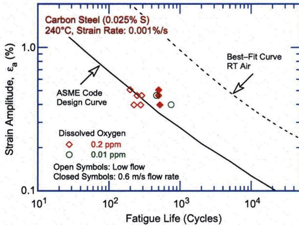
Figure 25. Effect of flow rate on low-cycle fatigue of carbon steel tube bends in high-purity water at 240°C (Ref. 44). RT = room temperature.
