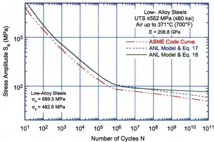
Figure 10. Fatigue design curve for low-alloy steels in air. The curve developed from the ANL model is based on factors of 12 on life and 2 on stress.
