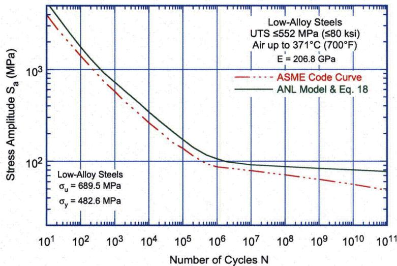
Figure A.2. Fatigue design curve for low-alloy steels in air. The curve developed from the ANL model is based on factors of 12 on life and 2 on stress.
