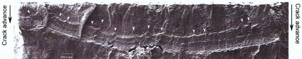
Figure 48. Crack front on Sample J11CC-1. Crack growth is from top to bottom.
