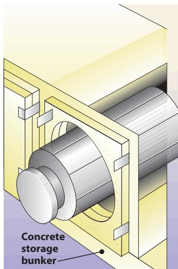
**2** The canisters can also be stored in above-ground concrete bunkers, each of which is about the size of a one-car garage. Eventually they may be transported elsewhere for storage.
