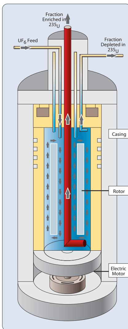
The gas centrifuge process uses a large number of rotating cylinders in a series and parallel configurations. Gas is introduced and rotated at a high speed, concentrating the component of higher molecular weight towards the outer wall of the cylinder and the lower molecular weight component towards the axis. The enriched and the depleted gas are removed by scoops.
