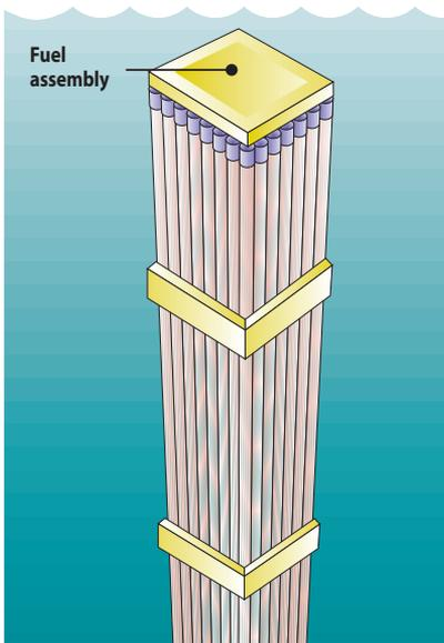
**2** After about 6 years, spent fuel assemblies — typically 14 feet long and containing nearly 200 fuel rods — are removed from the reactor and allowed to cool in storage pools for a few years. At this point, the 900-pound assemblies contain only about one-fifth the original amount of  $U^{235}$ .
