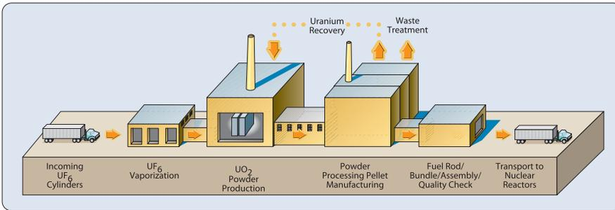
Fabrication is the final step in the process used to produce uranium fuel. It begins with the conversion of enriched uranium hexafluoride ( $UF_6$ ) gas to a uranium dioxide solid. Nuclear fuel must maintain both its chemical and physical properties under the extreme conditions of heat and radiation present inside an operating reactor vessel. Fabrication of commercial light-water reactor fuel consists of three basic steps:
