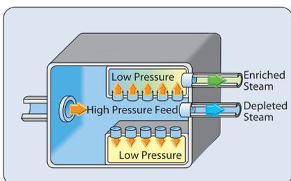
The gaseous diffusion method uses molecular diffusion to effect separation. The isotopic separation is accomplished by diffusing uranium, which has been combined with fluorine to form  $UF_6$  gas, through a porous membrane (barrier) and utilizing the different molecular velocities of the two isotopes to achieve separation.
