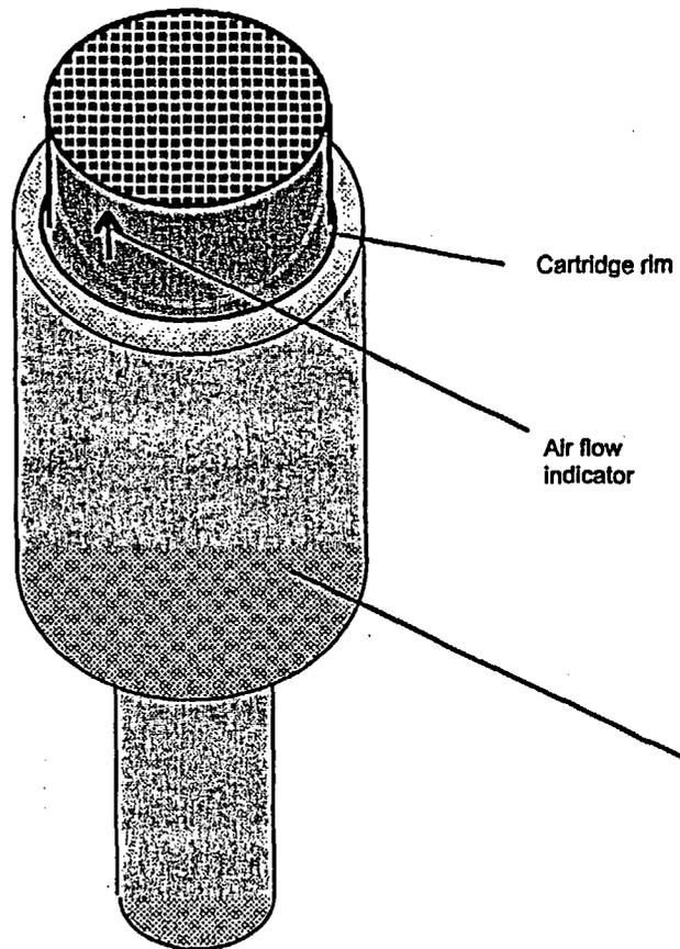
Figure 1. Face loading of the charcoal cartridge.
