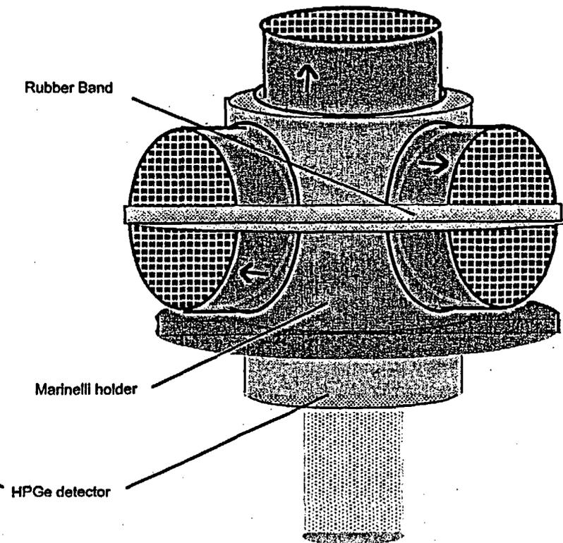
Figure 2. Face loading of cartridges in a batch.
